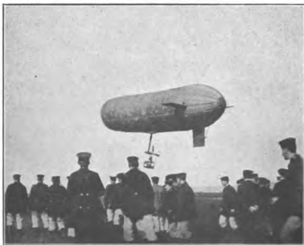
PARSIFAL AIRSHIP, showing one of the fixed horizontal planes, steering rudder, and car.
