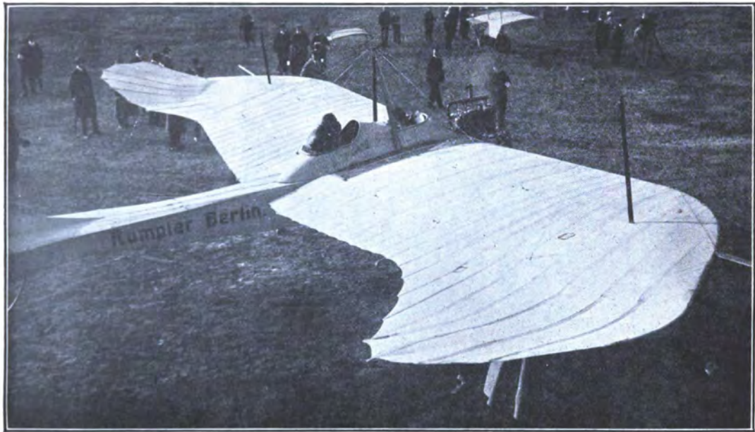
A RUMPLER MONOPLANE (A TAUBE), showing the distinctive bird shape so affected by the German monoplane makers.
