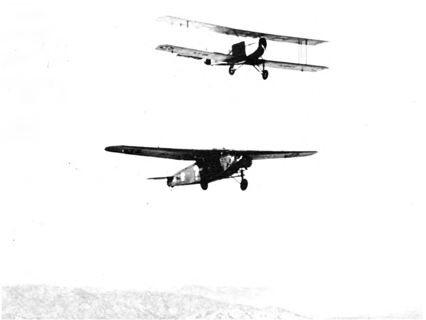
The Fokker C-2A, "Question Mark", being refueled by the Douglas C-1, during record endurance flight. (AF 46756AC)
