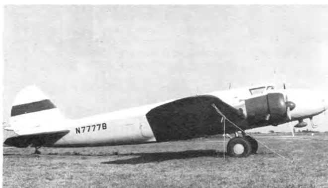
By the 1960s, c/n 1688 looked liked this, equipped with AT-6 cowlings and modified nacelles. (P. M. Bowers)
