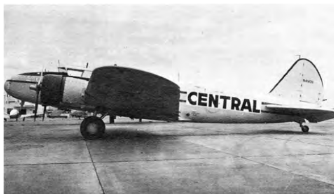
With trailing edge fittings for spraying work installed, c/n 1699 served Central Aircraft in the 1950s. (Bowers)
