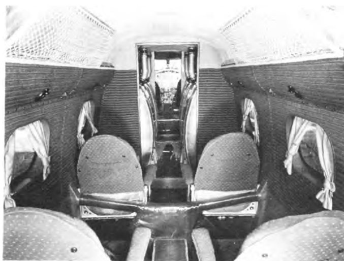
In foreground are four of the six seats in the rear cabin of the 247-Y, c/n 1952, and beyond are the four extra fuel tanks from Turner's plane. (Boeing #9378B)
