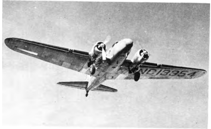
C/n 1736 serving Western Air Express in the late 1930s with spinners to avoid icing prop mechanism. (Bowers)
