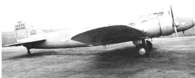
C/n 1686 carrying United shields of 1937-40 period with sealed off upper baggage door visible. (Williams)
