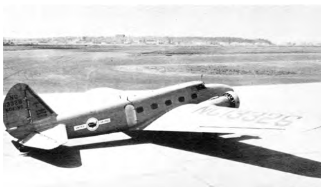
C/n 1707 with 247-D cockpit enclosure after a minor accident at Newark. Other 247-D changes made 2 yrs later.
