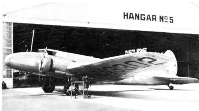
C/n 1683 with Boeing Air Transport. Pitch of 3-blade propellers was adjustable only on ground. (Bowers)
