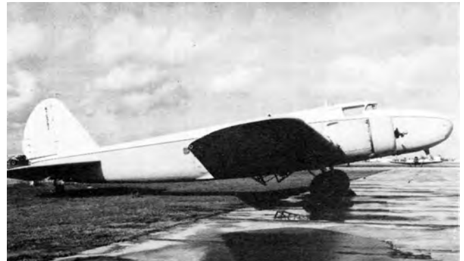
With BT-13 cowlings, extra windows and spray rig attached, c/n 1714 was used by Robertson Aviation. (Bowers)
