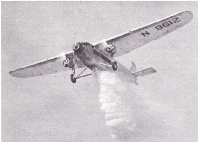
Ford 4-AT-E, N-9612, with a 300-gallon capacity was used in Montana in August 1957- N-8407 was also used during the same year. (Photo - U. S. Forest Service)
