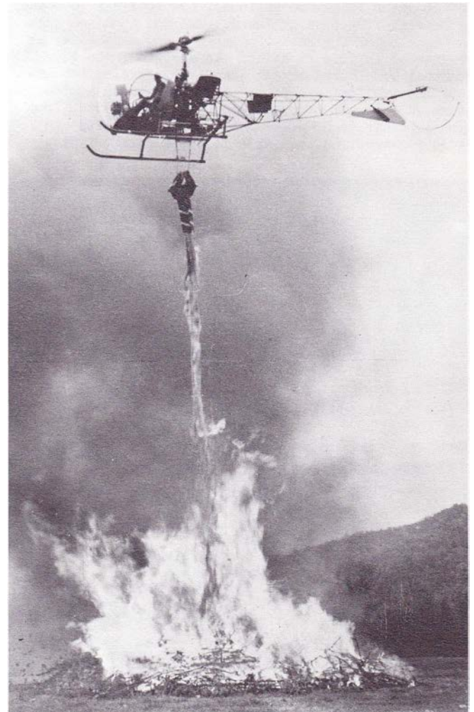
Bell 47 helicopter making a demonstration drop of 35 gallons of bentonite at Clark Tract, West Virginia, on 22 Oct 1959. (Photo - U. S. Forest Service 493131)
