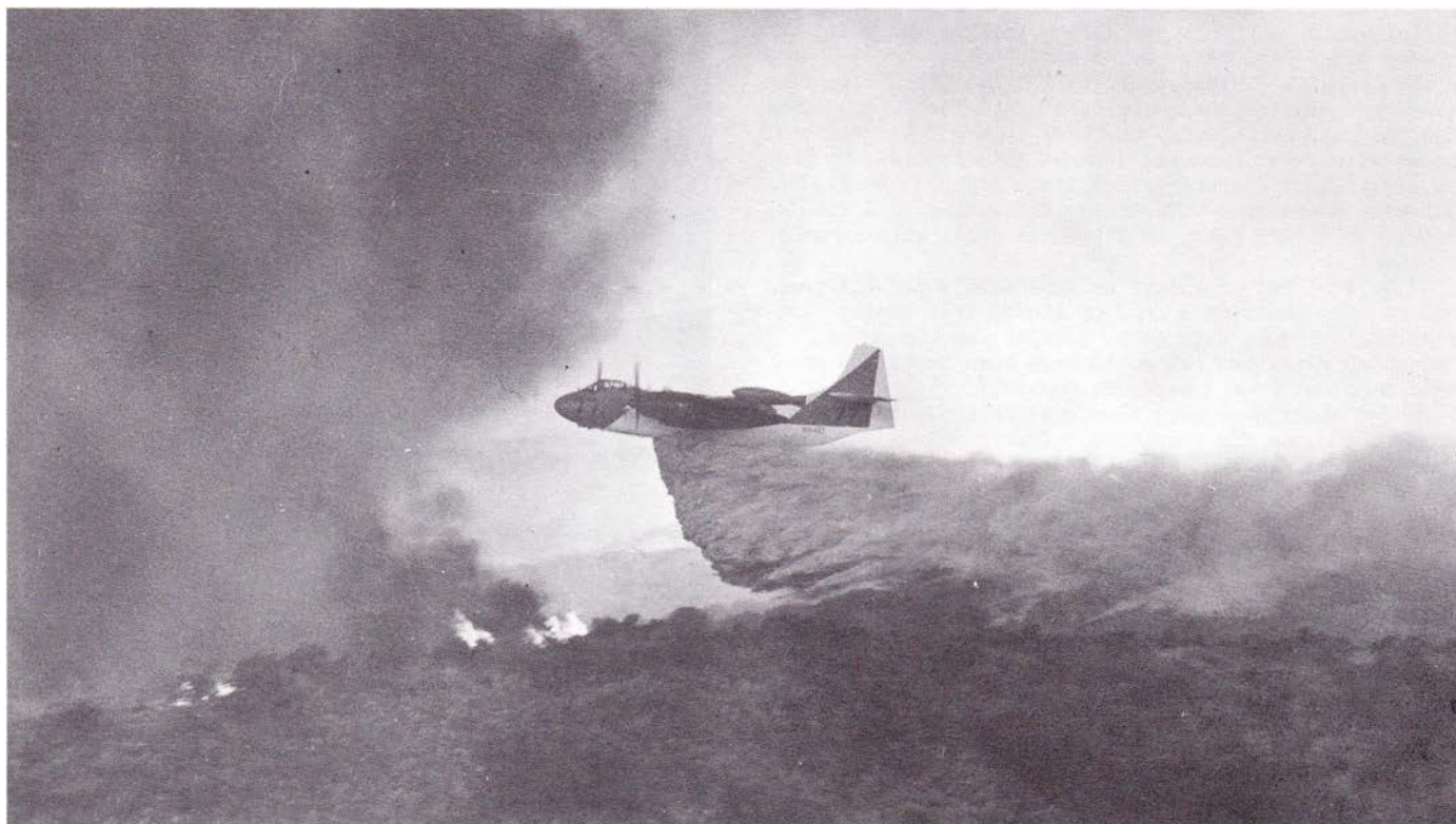
North American AJ-1, Number E 77, making a bentonite drop on a fire in Southern California. Intense smoke and lack of visibility are two of the major hazards in this type of flying. (Photo - L.A. Co. Fire Dept. 1867-19)
