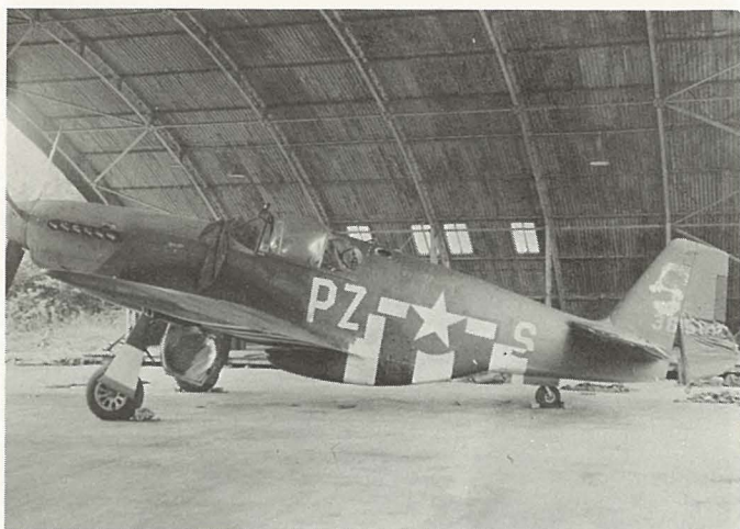
Hangared for repairs is PZ-S, 43-6500, with "displaced" lower rudder. Equipped with a Malcomb hood, it served with 486th Fighter Squadron of 352nd Group.
