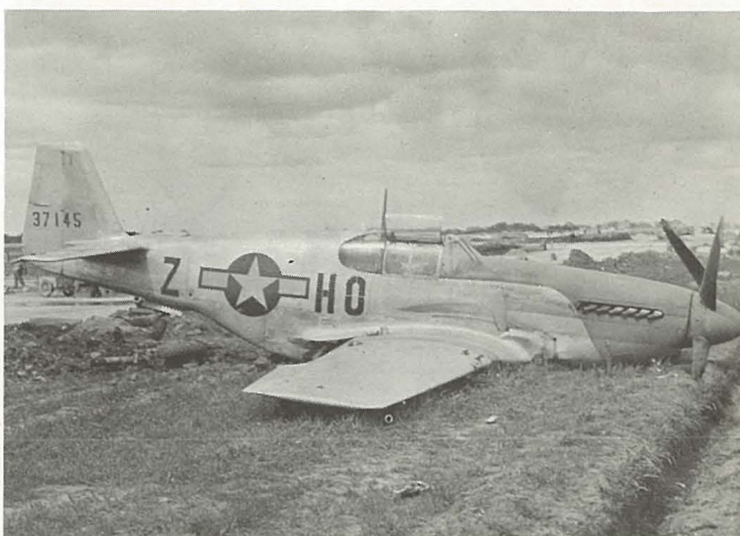
With distinctive blue nose of 352nd Fighter Group, HO-Z crash landed when engine cut-out on take off. The P-51B was with the Group's 487th Fighter Squadron.
