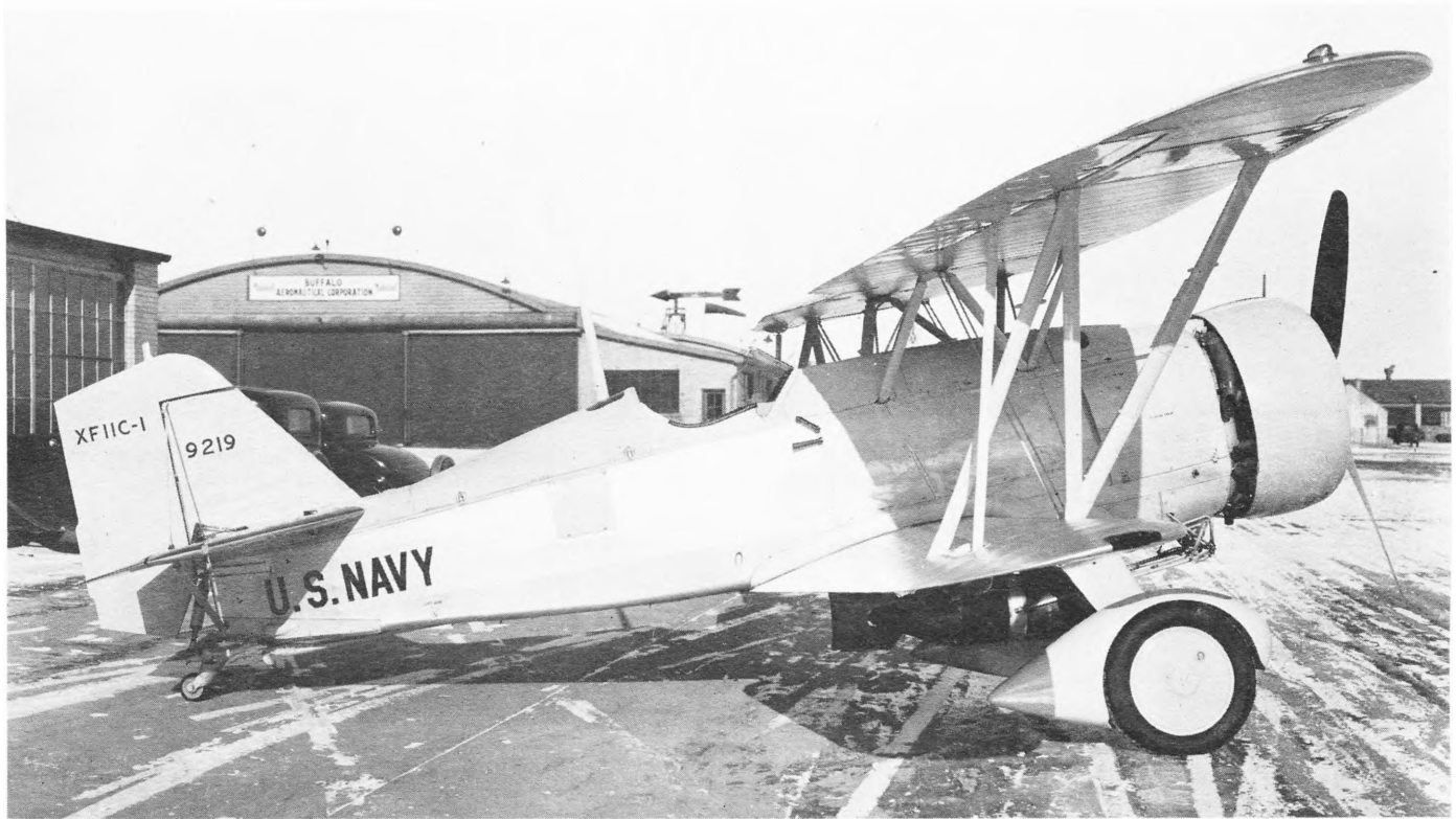
The Curtiss XF11C-1 at the factory with a 500-lb bomb attached to the bomb release mechanism which swung it down and forward to clear the propeller. Engine is a Wright R-1510, twin row, 14- cylinder. (Photo - Curtiss W-7918)
