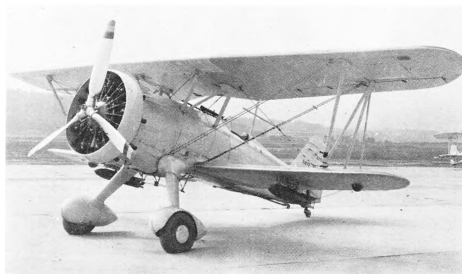
The same plane, number 9213, with 116-lb bombs underwing but with Wright SR-1820F engine and 3-blade propeller on July 19, 1932. (Photo - Navy AN-31562)
