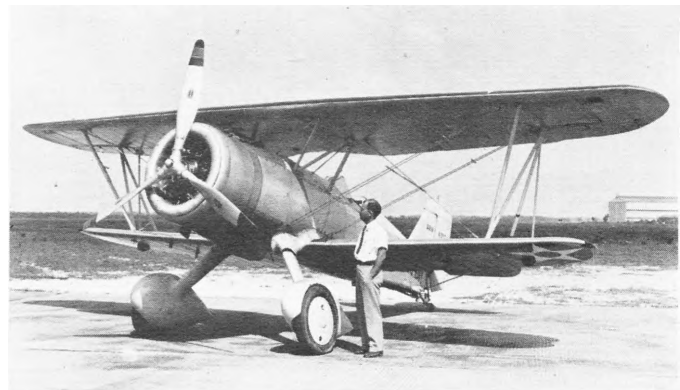
The XF11C-1 redesignated XBFC-1 and used to test various cowling configurations for better cooling at low speeds. At NACA Langley, 1936-38. (Photo - NACA LMAL 12063)
