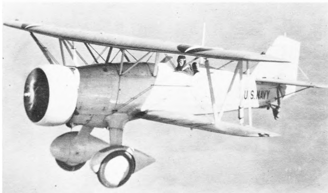
A rare flight photo of the XF11C-1 taken on November 4, 1932. Note the twin row engine, cowling, wheel struts and pants. (Photo - Curtiss W-7803)
