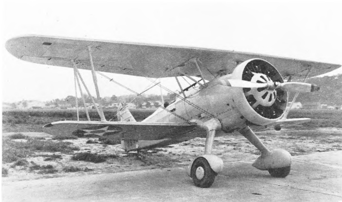
The Curtiss XF11C-2 in clean condition, without bombs or belly tank, is seen on May 17, 1932 with Wright R-1820-E engine and 2-blade propeller. (Photo - Navy AN-31554)
