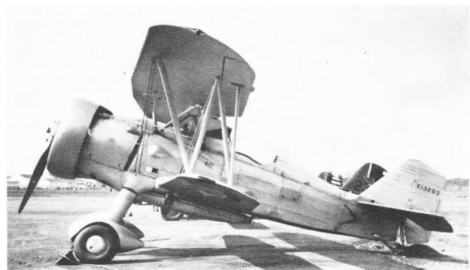
The civil demonstrator for export sales of the Goshawk, factory serial DH-46, was licensed 8-1-33. Note modified, flattened belly tank. (Photo - William T. Larkins)
