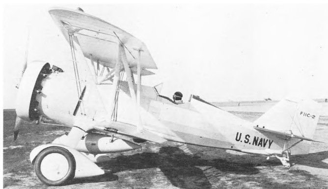
A Curtiss F11C-2 equipped with 50-gal. belly tank. During tests the XF11C-2 sustained 10.2 Gs on pullout, the highest ever recorded for a Naval aircraft. (W-7788)
