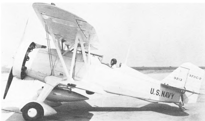
The XF11C-2 with distinctive small air wheels and pants, thin cowling, radio mast, etc. is seen at the factory on June 22, 1932. (Photo - Curtiss W-7457)
