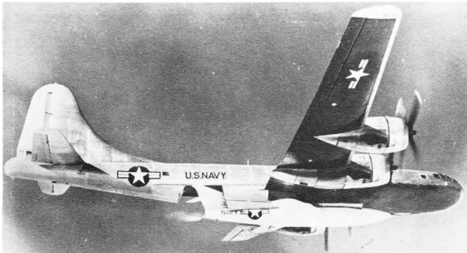
The P2B-1S, 84029, was modified to carry the Douglas D-558 research aircraft aloft to be air launched for rocket-powered flight. (Photo - Boeing)
