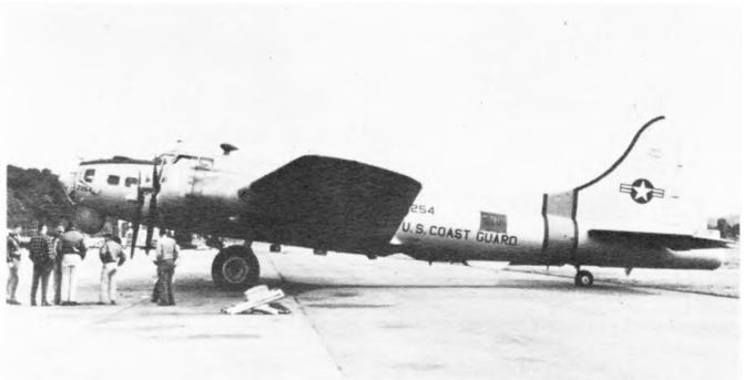
77254 was specially equipped with nine lens camera (at lower rear of fuselage) and was used by the Coastal and Geodetic Survey for aerial mapping. (Photo - Boeing)
