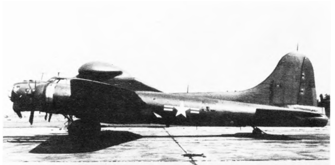
Bureau Number 77234 is seen in September 1950 with a later development in the PB-1W series, overhead carriage of the radome which proved more efficient. Few PB-1Ws were modified. (Photo - Hal Andrews)
