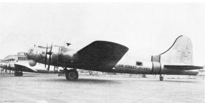
This PB-16, 77255, was equipped for Ice Observation duty on International Ice Patrol and is seen awaiting take off from Argentia, Newfoundland. (Photo - USCG)
