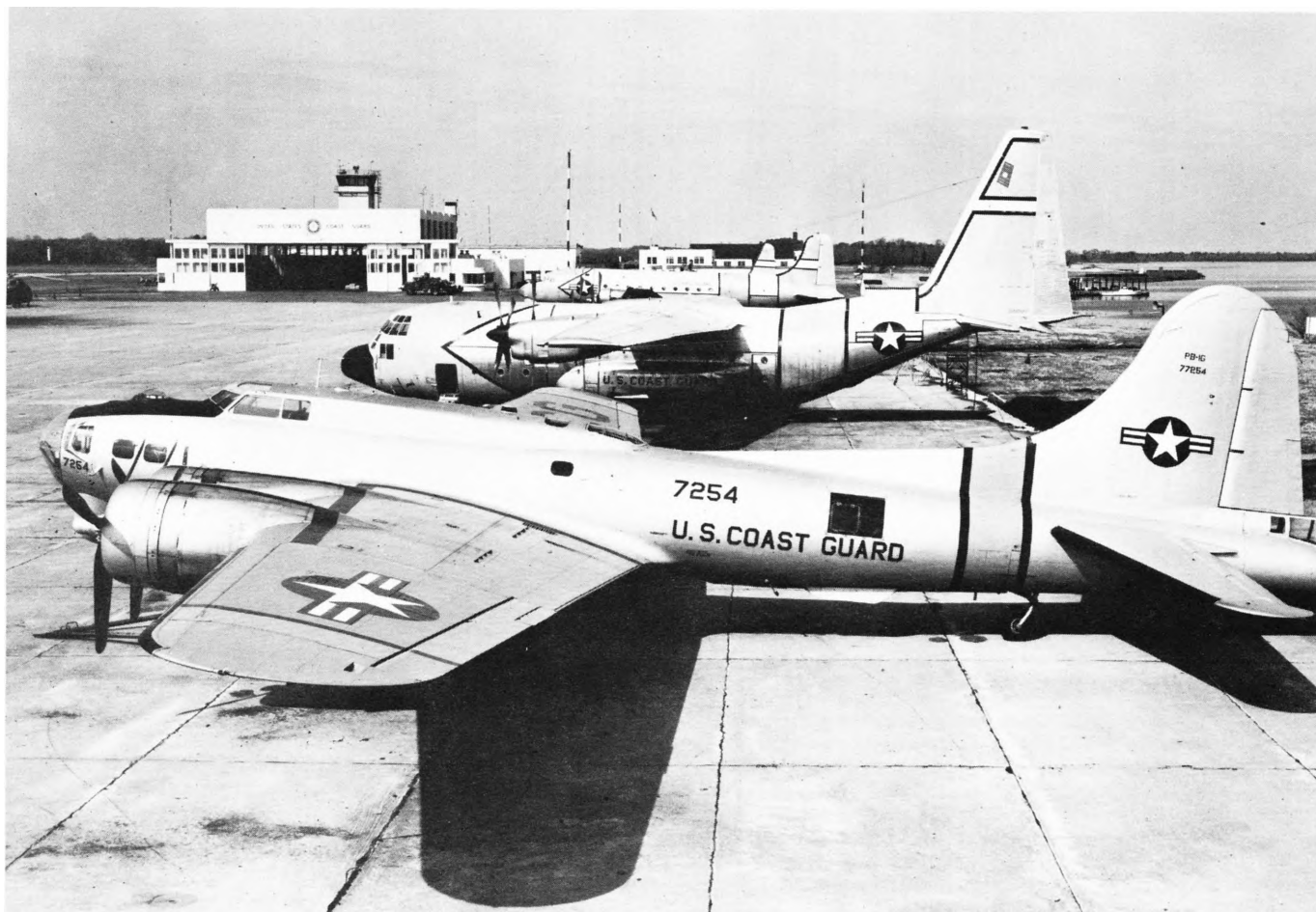
This Boeing Flying Fortress PB-1G, Bureau Number 77254, served, fourteen years with the Coast Guard as a special photo plane. The C-130B in the background accepted January 12, 1960 and marked the first use of turbine propulsion in U. S. Coast Guard aviation. (Photo - United States Coast Guard)
