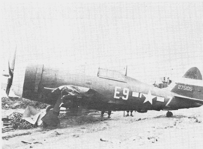
A Republic P-47D-10-RA, E9-Z, of the 376th Fighter Squadron, 361st Fighter Group showing the results of a forced landing on an uncompleted runway.
