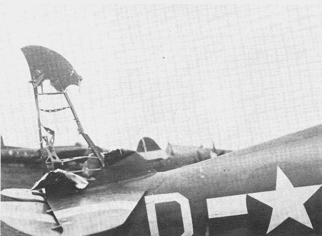
How much could a Thunderbolt take? This P-47D came home on aileron control only, after flak all but removed her vertical tail during a mission over Germany.
