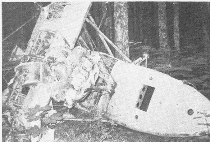
Another view of c/n 904 showing how the attentions of a bulldozer almost pushed the engine into the pilot's compartment. (Photo - Phil Redden)
