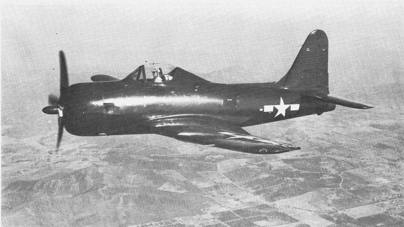
With a dorsal fin slightly modified from the final configuration, the second XFR-1, BUONO 48233, is seen during a test flight over San Diego. The clean lines of the aircraft are quite evident. (Photo - Ryan 28-1680)
