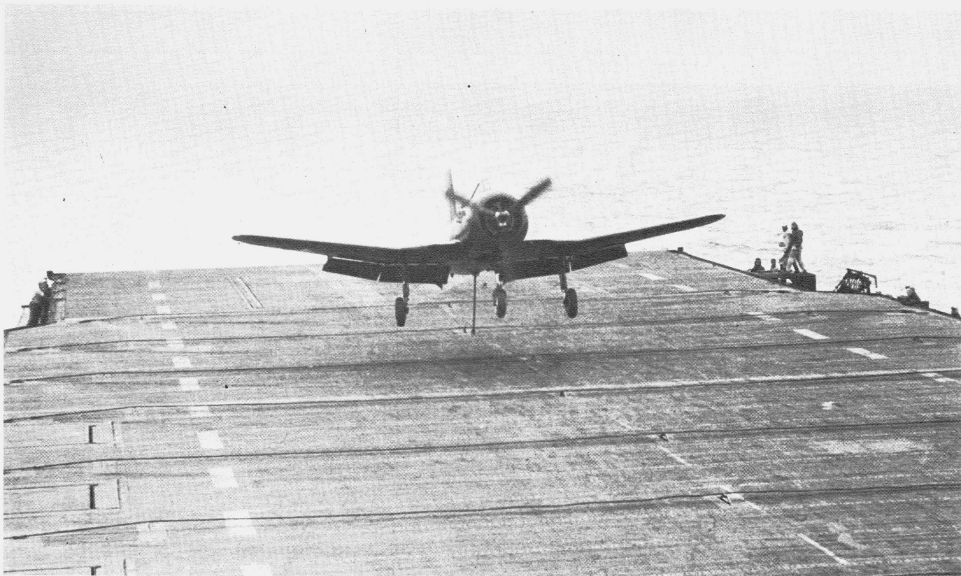
A Fireball comes in nose high with hook extended and reaching for arresting wires during the qualification trials on board the USS Ranger, run during the first days of May 1945. (Photo - Ryan 28-4754)
