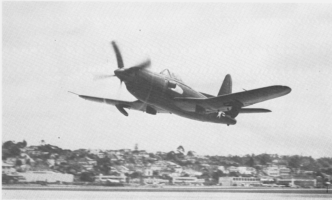
Airborne on its first flight is the Ryan XF2R-1 Dark Shark, BUNO 39661, taking off from Lindbergh Field, San Diego, California. Main difference from the FR-1 was the turboprop engine. (Photo - Ryan 29-102)
