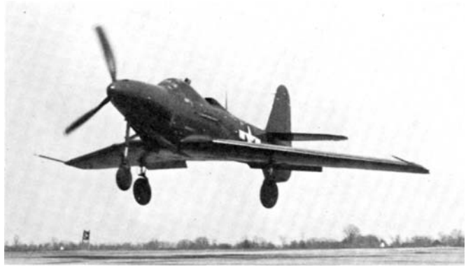
Note 3-bladed propeller obtained from P-39Q-10s on U.S. Navy L-39, swept wing P-63 conversion. (Bell 73114)
