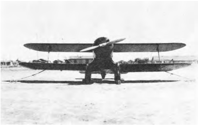
The narrow landing gear is very evident in this view of C/N 2. Note the landing lights above the wheel spats and the second phase cowling. (Photo - E. F. Ross Collection)
