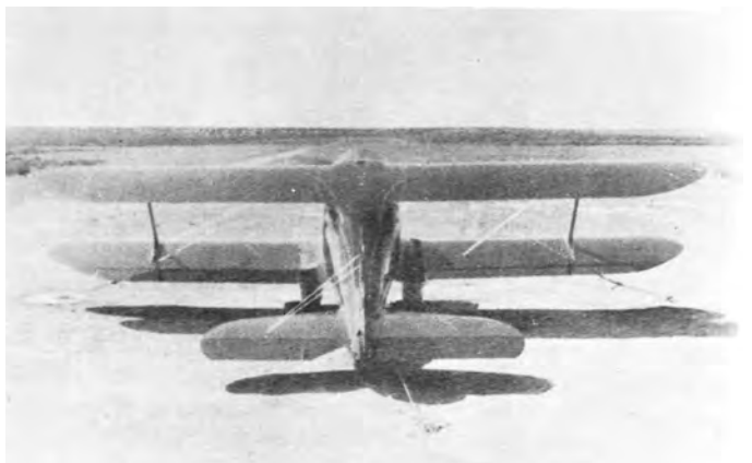
The rear view of C/N 2 with empennage bracing wires. These broke several times in flight and Eddie Ross suggested the change to steel tubing, which was used on all later Staggerwings. (Photo - Ross Collection)
