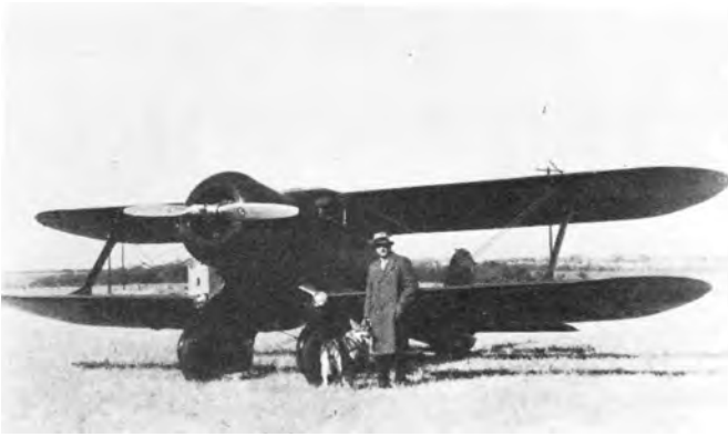
Probably C/N 1, since this photograph appeared in AERO DIGEST Magazine of December 1932 prior to the time that C/N 2 was built. It then had an NACA type engine cowling. (Photo - Peter M. Bowers Collection)
