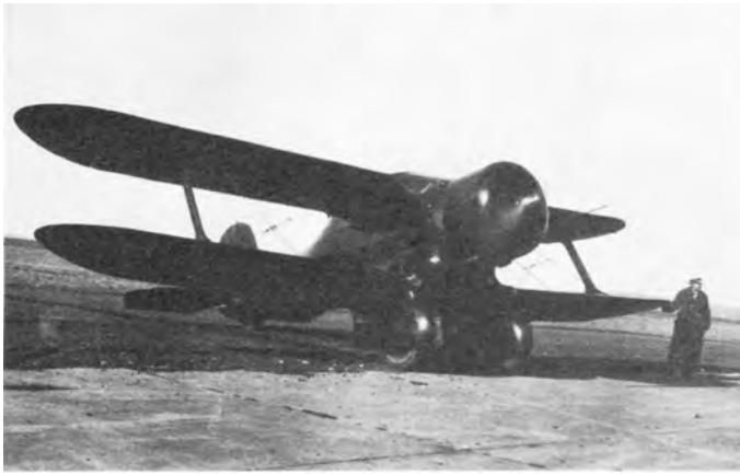
Another view of C/N 2 in which it is possible to just make out the fairing around the fixed tailwheel. (Photo - Ross Collection)
