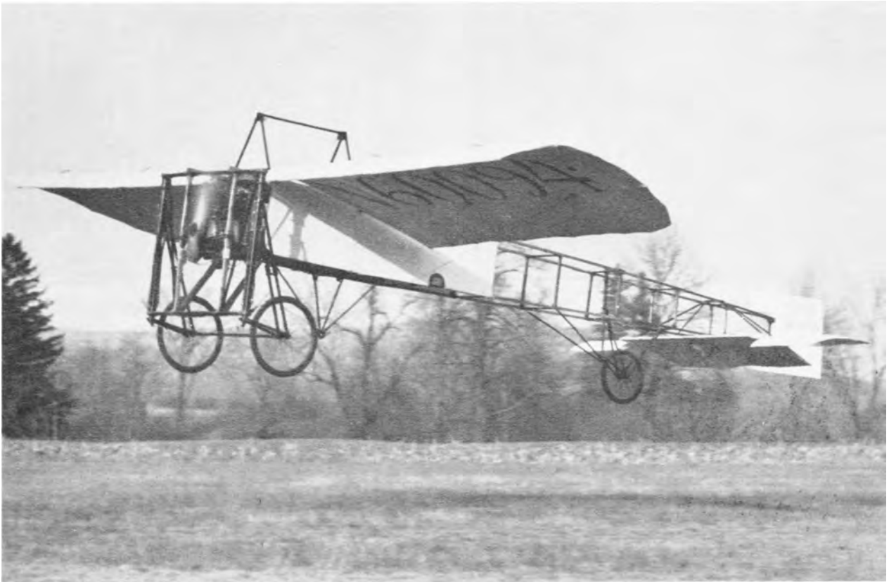
Cole Palen's restored Bleriot XI, Number 56. The engine was installed in the rear of the "bedstead" at this time. Also the position of the tip elevators is very pronounced.
