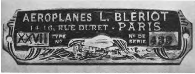
The nameplate for Bleriot XXVII, Serial Number 453, from the Nash Collection. Brass with raised, polished letters and black background. Original width 3".
