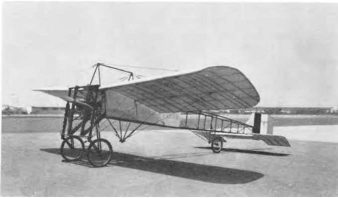
The Provolt-Weeks Bleriot XI, 2s, with a 45 hp Continental engine as used in the motion picture LAFAYETTE ESCADRILLE. (Photo - Ed Maloney)
