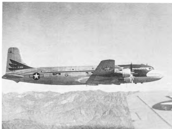
Nose contour of the INDEPENDENCE was changed by APS-10 radar. Three windows indicate position of Presidential stateroom. (Photo - Douglas 85-11-1)
