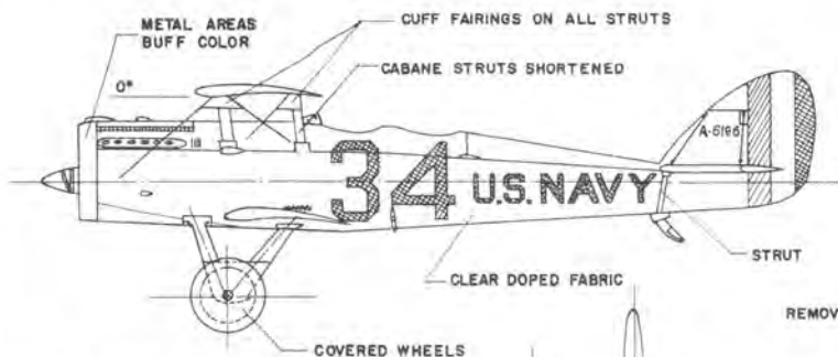
DH-4B-3 RACING PLANE PACKARD 2A-1500, V-12 ENGINE 600 HP AT 2500 RPM
