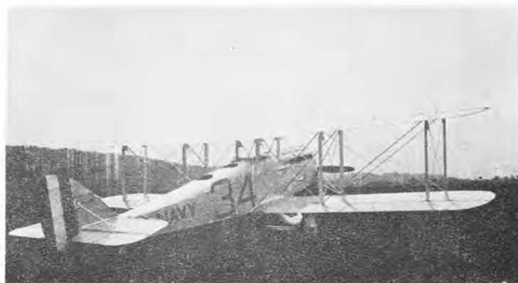
DH-4B-3 entered by Navy in the 1927 Curtiss Race at Curtiss Field, L.I. and to be flown by Capt. F.O. Rogers, USMC. It crashed on the way to the Race. Packard 2A-1500 engine. (Photo - USMC, DOD No. 529389)
