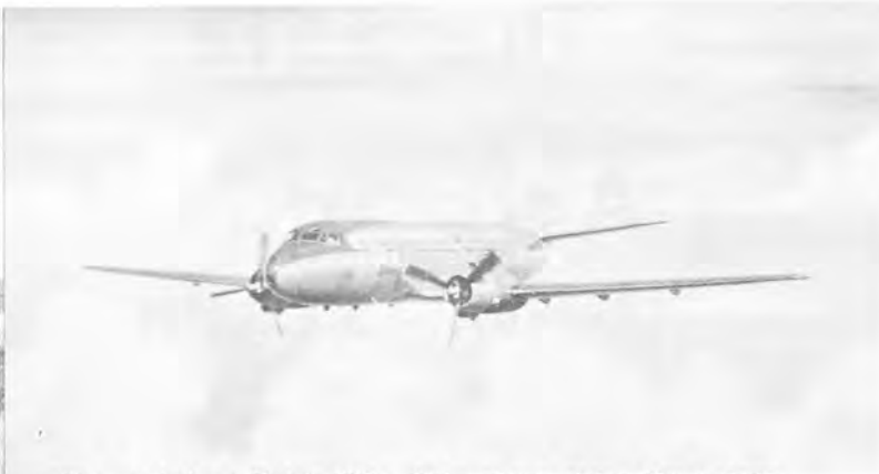
The prototype Model 202. This views shows the nearly straight wing. Vertical fin carries NX93001. (Photo - Al Roshkind)
