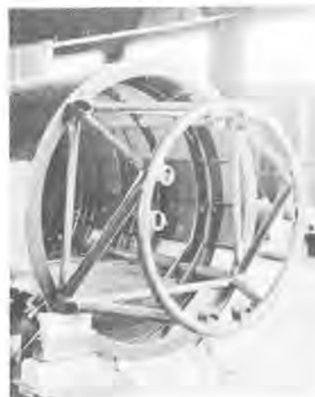
In 1937 it became more powerful with "Twin Wasp Jr." new mount, Northrop A-17A cowl. (Photo-C.F. Reynolds)
