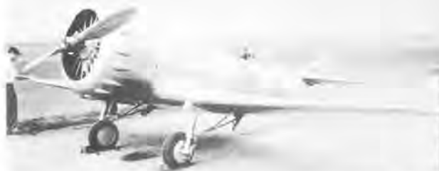
Ortman replaced the engine with a direct-drive "Wasp" for the 1935 Bendix Race. (Photo - C.G. Mandrake)
