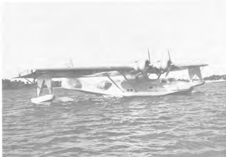
UH-EAX was operated by Qantas over the Australian-Pacific Islands on regularly scheduled service from 1947. It had two Pratt & Whitney R.1830-92 engines of 1050 H.P. and cruised at approximately 120 mph. In long flights it could carry 28 passengers and for the shorter New Guinea operations its high density loading was 44 passengers. (Photo - Qantas)
