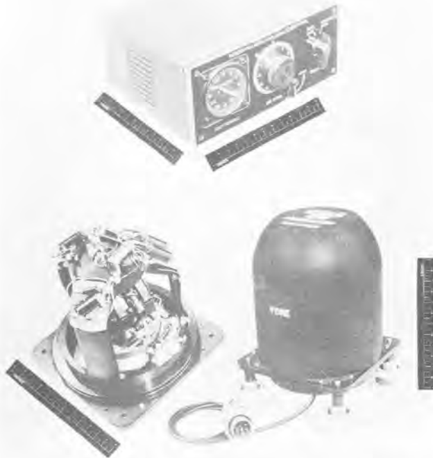
Gyro Flux Gate Compass. This instrument, developed by Pioneer Instrument Co., was eventually installed on most military aircraft and provided the most accurate direction-indicating device up to WWII. (Photo - Eclipse - Pioneer Div., Bendix Corp.)
