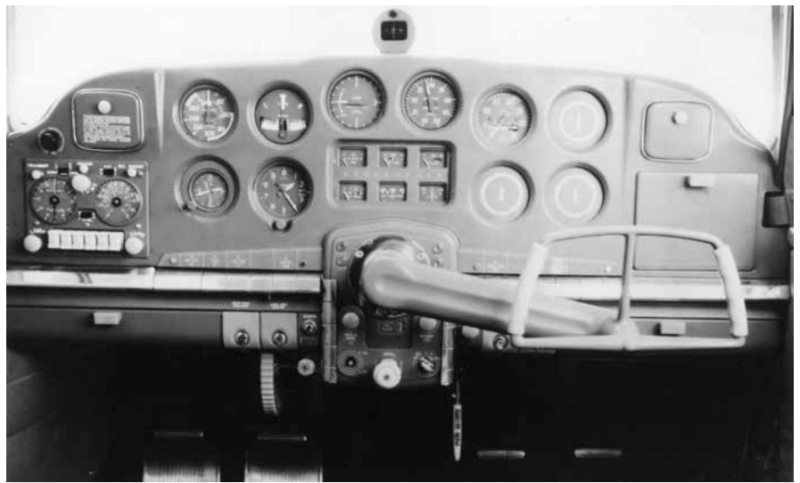
Original instrument panel, complete with gyroscopic turn-and-bank indicator and radio. Throw-over control wheel aided comfort for the non-piloting person in front. Defying tradition, Harmon went for a bluegray panel to differentiate instruments and blend with the sky. There would be no black in the cabin.[Harmon] (AAHS archives, Gerald Balzer collection)
