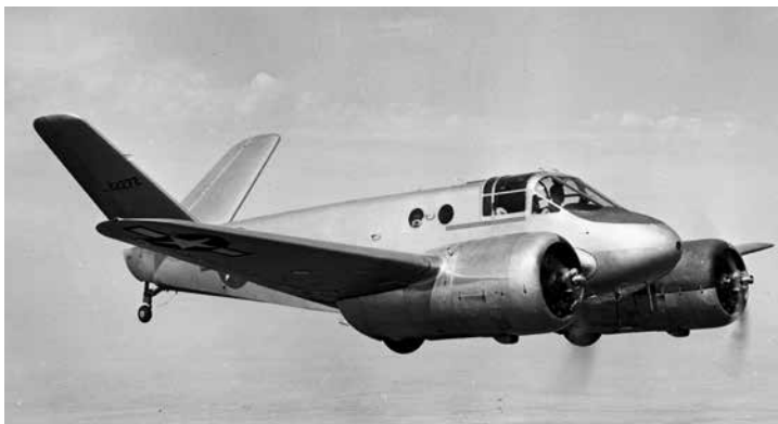
The Beech AT-10 twin-engine trainer, modified with a V-tail, showed a 3-mph boost in speed, and no particular vices. (AAHS archives, Gerald Balzer collection)
