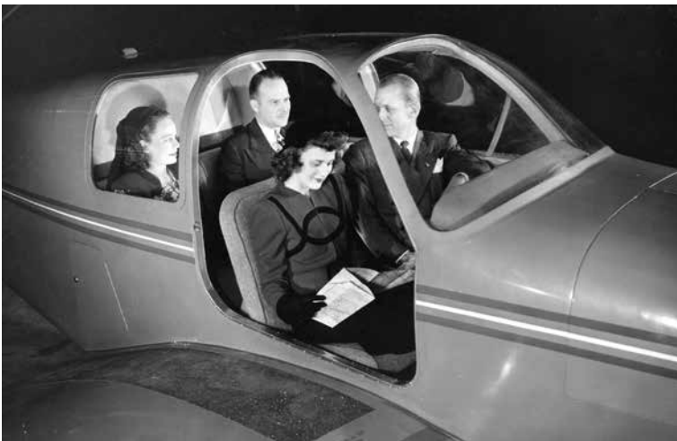
Four seats, in automotive comfort, even for the ladies. Big door simplified entry and exit. Note exterior baggage hatch. Integral roll-cage structure protected occupants. Flush windshield cut drag. Big windows aided visibility and comfort. (Beech photo, AAHS archives, Gerald Balzer collection)
