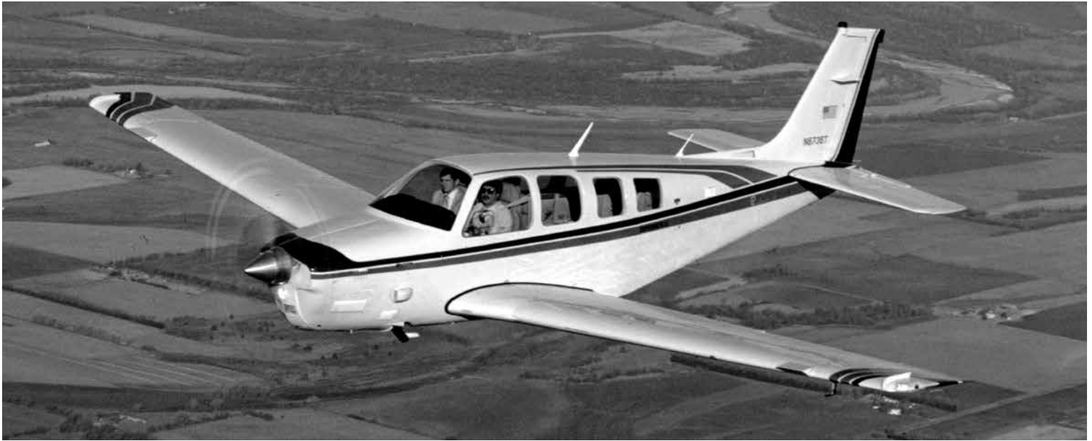
B36TC, the ultimate Bonanza: 300 hp, 245 mph top speed at 19,000 feet. 230 cruise at 25,000. Extended wings hold fuel for 1,133 miles at 196mph. Full-fuel payload: 878 lbs;[B/T;D/B] (Beech photo, AAHS archives, Gerald Balzer collection)
