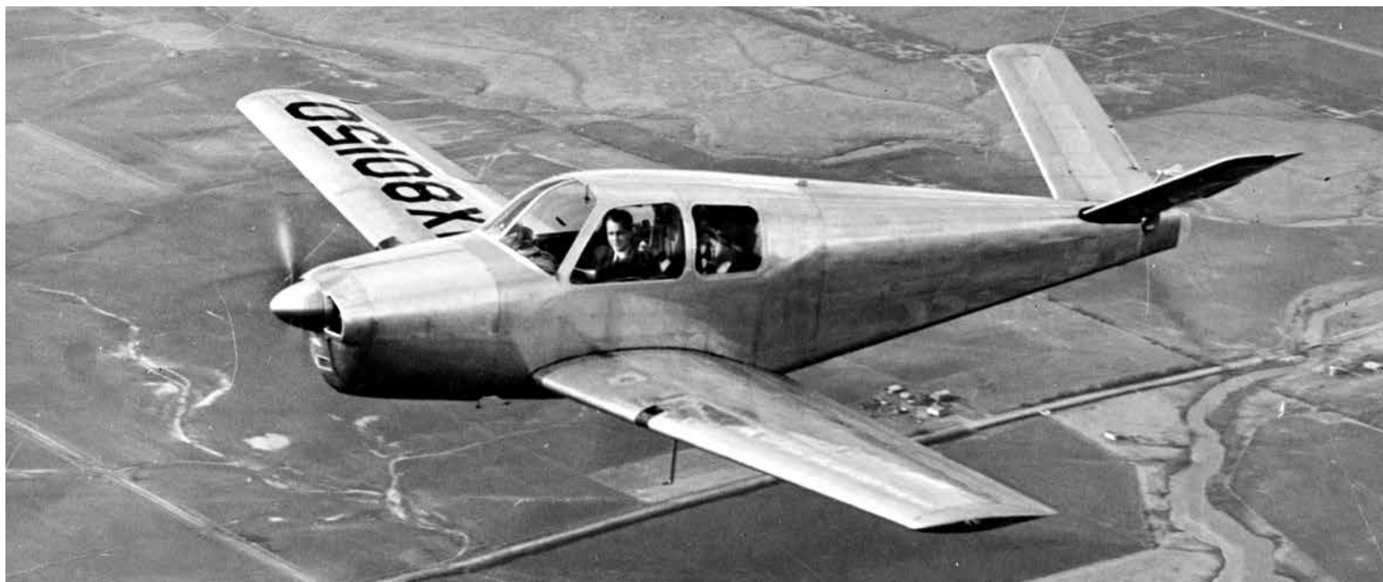
Prototype #3, NX80150, with the laminar flow wing and Lycoming power. Believed to have been lost in flight testing due to a failure of the gear door during a dive. (Beech photo, AAHS archives, Gerald Balzer collection)
