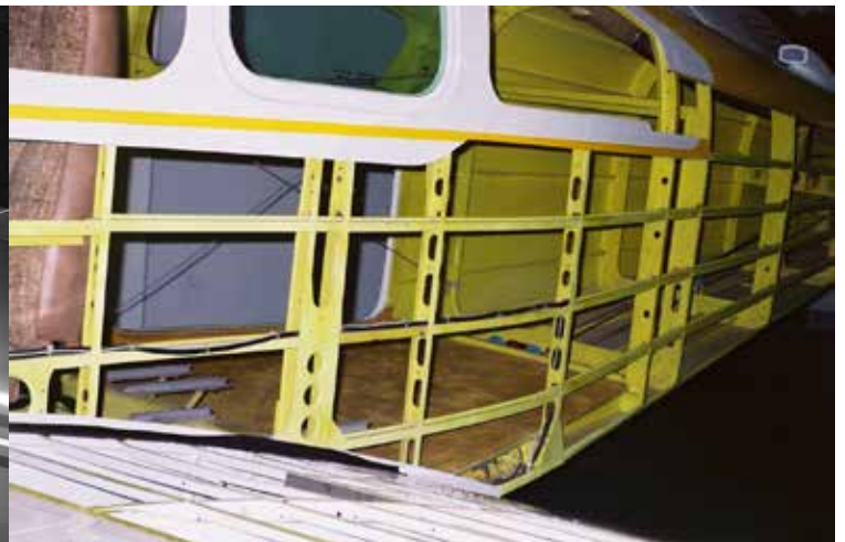
The 1st successful, fully modern light plane used modern semi-monocoque design: A hollow aluminum shell, reinforced with vertical formers and horizontal stringers for light-but-strong, durable construction. (author's photo)
