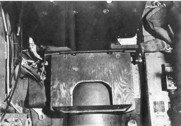
The small seat for the photographer in the rear is in the center of this view, and the modification apparently used a modified armor plate as the backrest. There were only small control boxes for the cameras on the starboard side, just visible at lower left and a basic safety belt. (RG18 NARA)
