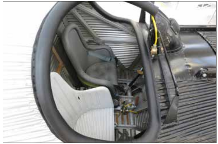
While the passengers enjoy a degree of comfort, pilots still sat in an open cockpit protected marginally by a small windscreen. Seen here is a slightly later model F-13 (circa 1923) that still retains the open cockpit design. (Photo via Flickr by Pilot_Micha)
