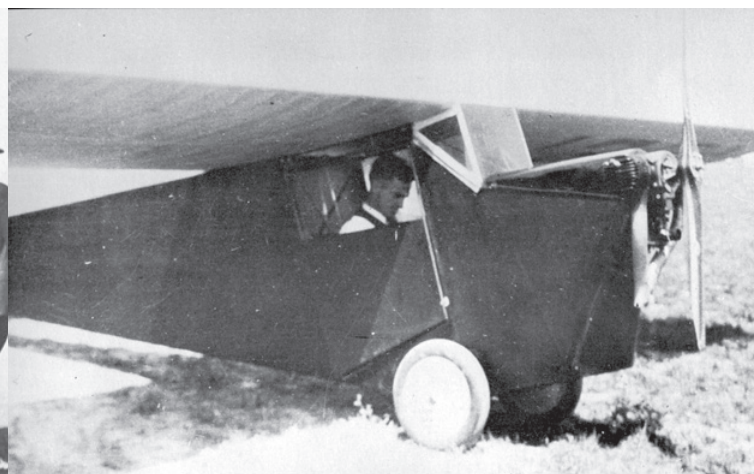
Eldon Cessna created the "Baby Cessna" by wrapping the CS-2 frame in a fuselage and a tiny enclosed cabin, adding wheels and a 25-hp Cleone engine.
