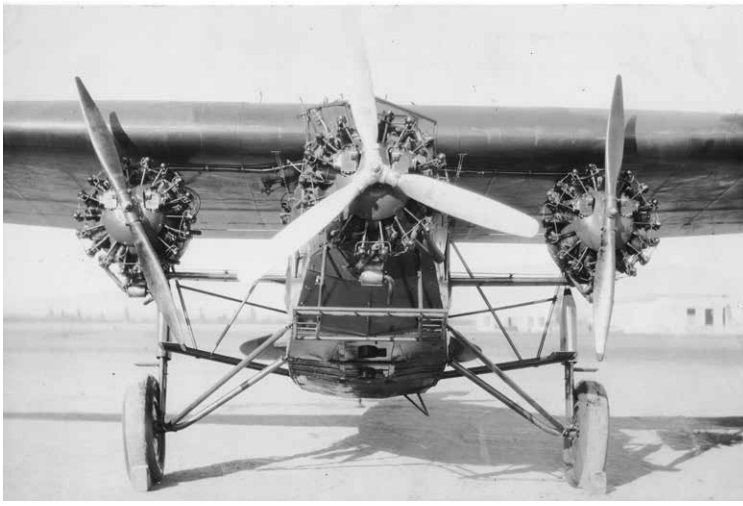
The position of the engines is shown in this front view of C-2A, 28-120, 'Question Mark', the most famous of the type. The trapezes to service the engines during the endurance flight early in 1929 are visible.
