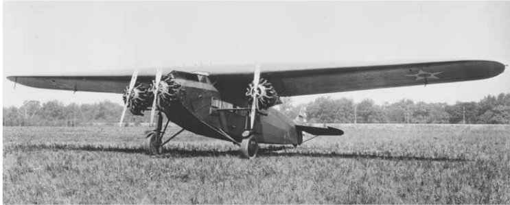
The 28-126 as modified on Wright Field to take the new Wright R-975 engines and redesigned as XC-7 with tail number XP545.
