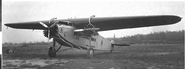
The US Navy was the first to fit a three-blade propeller on the type, as shown in this photo at Anacostia, D.C.
