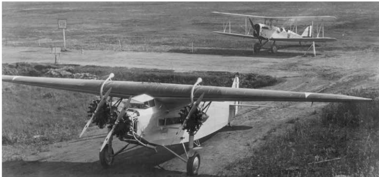
The first TA-1 Trimotor for the U.S. Navy at the factory, still with its two blade propellers.
