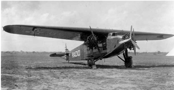
The Air Corps second C-2, 26-203, as modified for radio experiments. Note the three-blade nose propeller.
