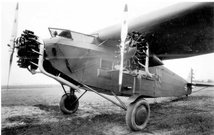
The first Air Corps C-2A, 28-119, completed as third of the improved Trimotors, easily being recognized by the larger wing with the rectangular center section.
