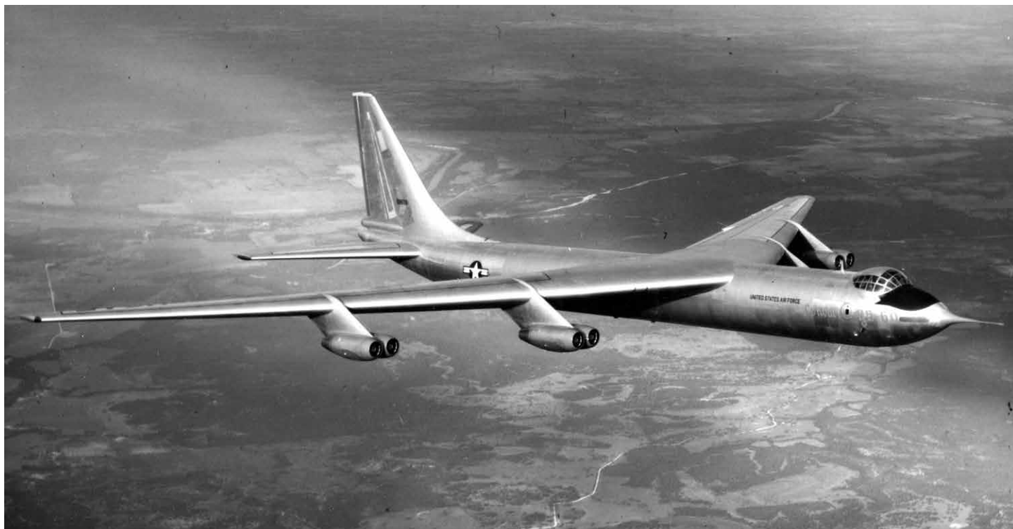
The YB-60 basically combined a B-36 fuselage with new swept wings and empennage surfaces and eight turbojet engines. The needle nose contained test instrumentation. (AAHS-d023067 from the NARA collection)
