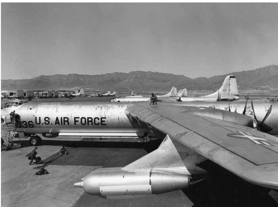
B-36B 44-92036 with the installation of General Electric J47 engines. The nacelles had shutters to close the inlets and eliminate windmilling drag when the engines were not in use. (AAHS-D023947 from the NARA collection)
