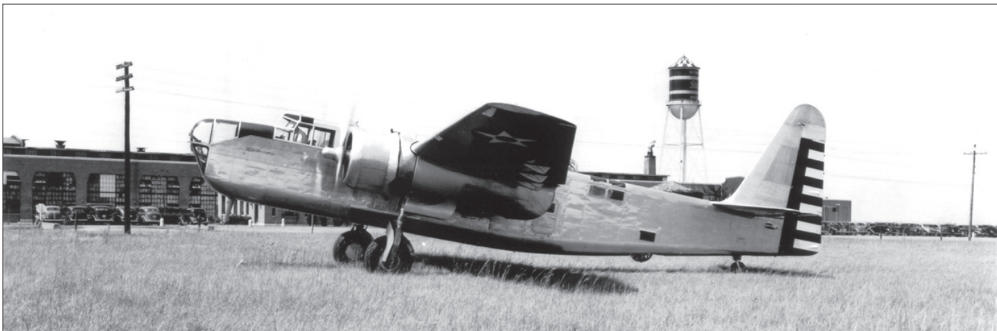
The modified “stepped” cockpit configuration shows well in this photo of the XA-21 parked in the grass at the Stearman factory. (Stearman Aircraft Co. photo from the Kenneth D. Wilson collection)
