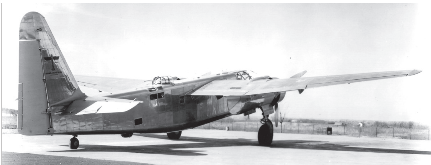
Right rear view clearly shows the gun turrets on the upper and lower fuselage. (Stearman Aircraft Co. photo from the Kenneth D. Wilson collection)
