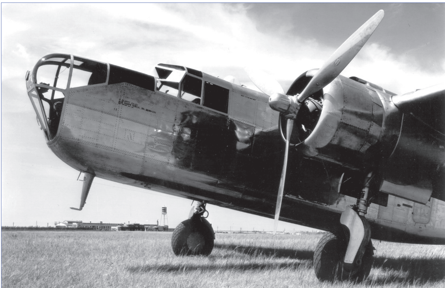
Good view of the modified "stepped" cockpit configuration and the engine installation. The Stearman factory is in the background. (Stearman Aircraft Co. photo from the Kenneth D. Wilson collection)
