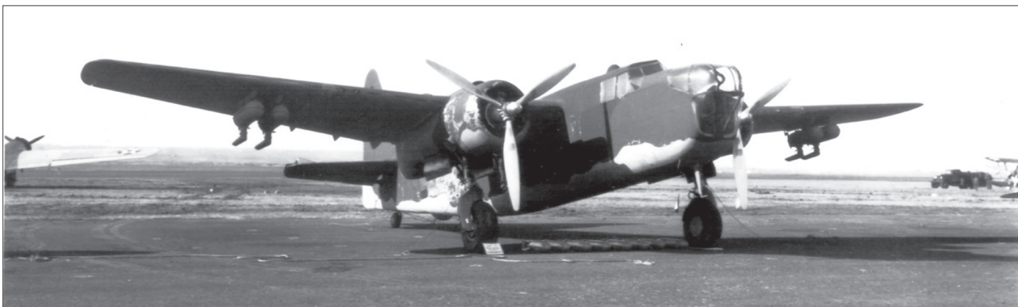
The Stearman XA-21, sporting a war camouflage paint scheme, on display at Wright Field in 1940 or 1941. Note the four chemical smoke generators on under wing racks. (U.S. Army Air Corps photo from the Kenneth D. Wilson collection)
