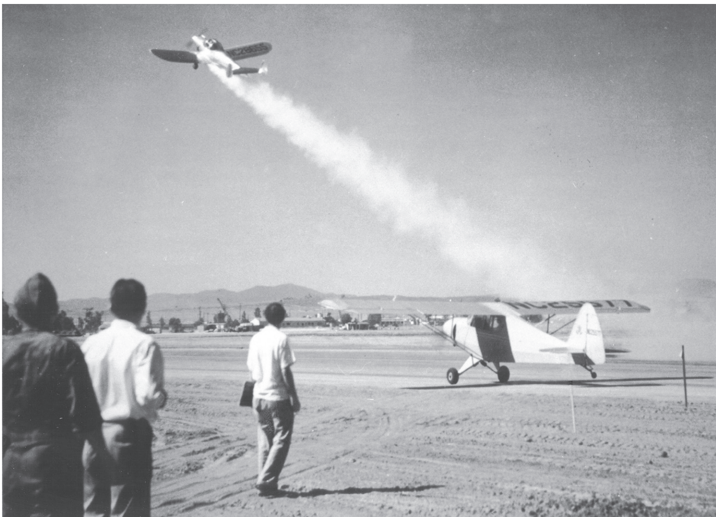
Ercoupe aircraft on a steep ascent with the help of JATO rocket. The pilot was Homer Boushey. (Photo from NASA Jet Propulsion Laboratory)
