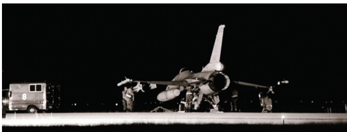
After flying morning CAPs loaded with only 20mm TP, followed by 20mm HEI in the afternoon, live AIM-9Ls missiles were delivered to the 113th ad hoc alert ramp on Taxiway Echo. Weapons loaders are seen here loading those AIM-9Ls on 85-481. (Photo by Michael Porter)
