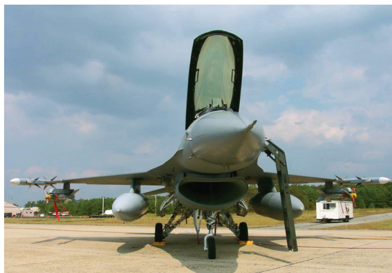
A 113th Viper parked on Taxiway Echo awaiting its next CAP sortie. Its configuration of two AIM-120s and two AIM-9s has since become the standard ACA weapons configuration. Photo: 113th PAO
