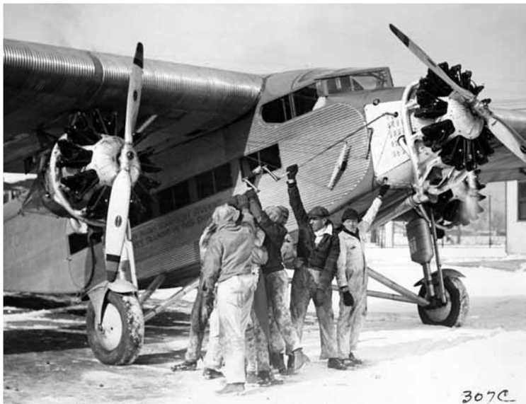
In the winter of 1929, these Parks Air College students are hand cranking the inertial starter for the Pratt & Whitney Wasp engine on the Ford Tri-Motor.
