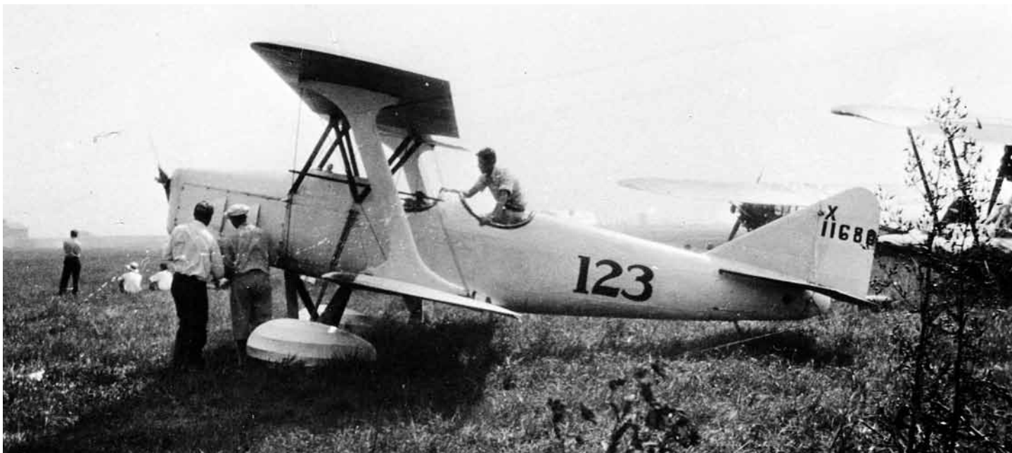
The Trainer Model 2 was transformed with the addition of the inline engine and wheel pants as X-11680 with the 85-hp Ford V-8 installed in a tidy cowling. The date of this image is uncertain but must have been after December 16, 1937. (via David W. Ostrowski)
