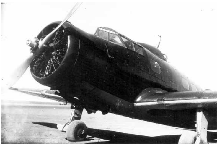
Close-up of one of the three Vultee V-1As that were converted into bombers by the Spanish Republicans at the Leon base. These planes were armed with two machine guns in the wings and bomb racks under the wings. (Photo from the Juan Arraez Cerda collection)
