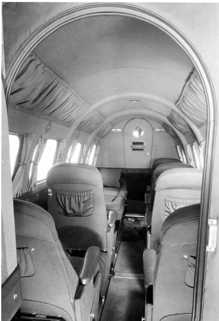
The cabin of the Vultee V-1A was particularly neat. The wing spar, placed very far forward, did not block the passage of passengers as on the Boeing 247. (Photo from the Gerald Balzer collection, AAHS)
