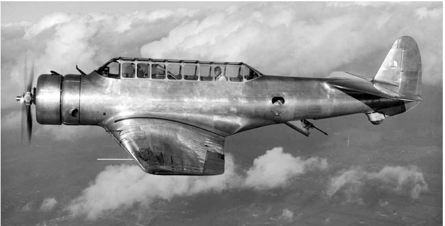
Using the same wing and some other available sub-assemblies, the engineers at Vultee's design office created a family of military aircraft to meet potential needs such as this V-11GB that one would hardly believe came from a commercial aircraft. (Photo from the Gerald Balzer collection, AAHS)
