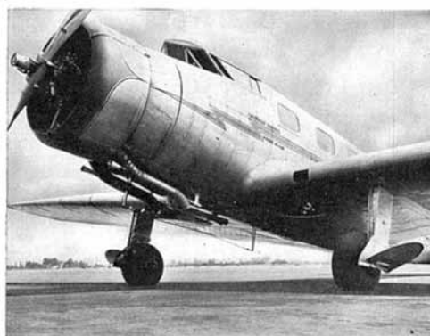
The new high-speed Vultee, built by the Airplane Development Corporation, has Airwheel Tires and Tailwheels, as well as Airwheel Hydraulic disc brakes
