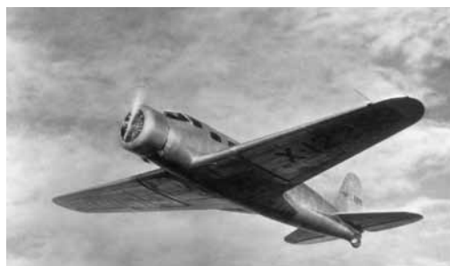
With few appendages that could disrupt the airflow around the airframe, the V-1A was one of the most modern airliners of its time. (Photo from the P.M. Bowers collection)
