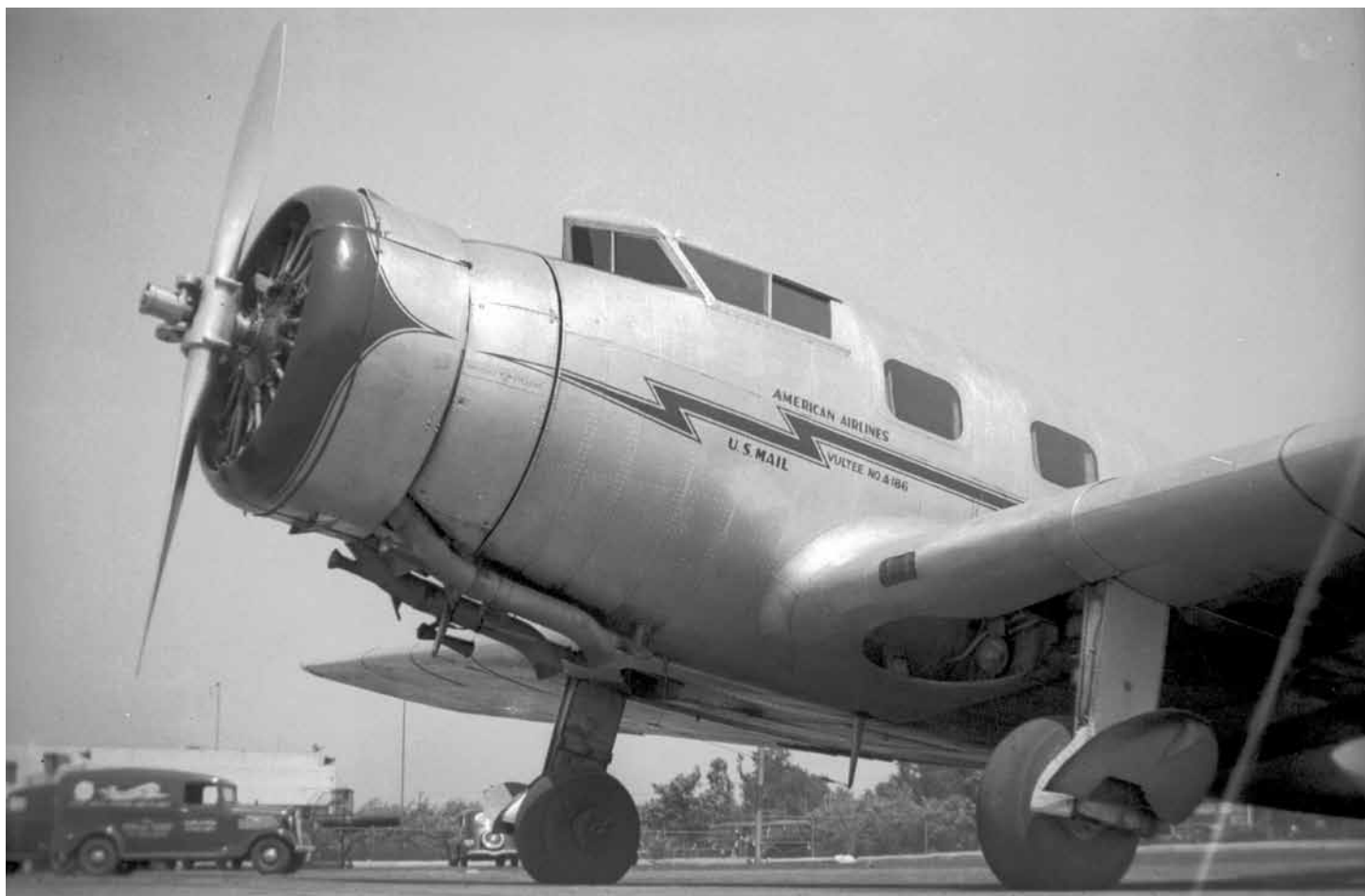
This close-up of an American Airlines V-1A shows many interesting details such as the landing light in the landing gear well, the sliding side window and the three-bladed variable-pitch propeller. (Photo from Rayburn Ray collection, AAHS)
