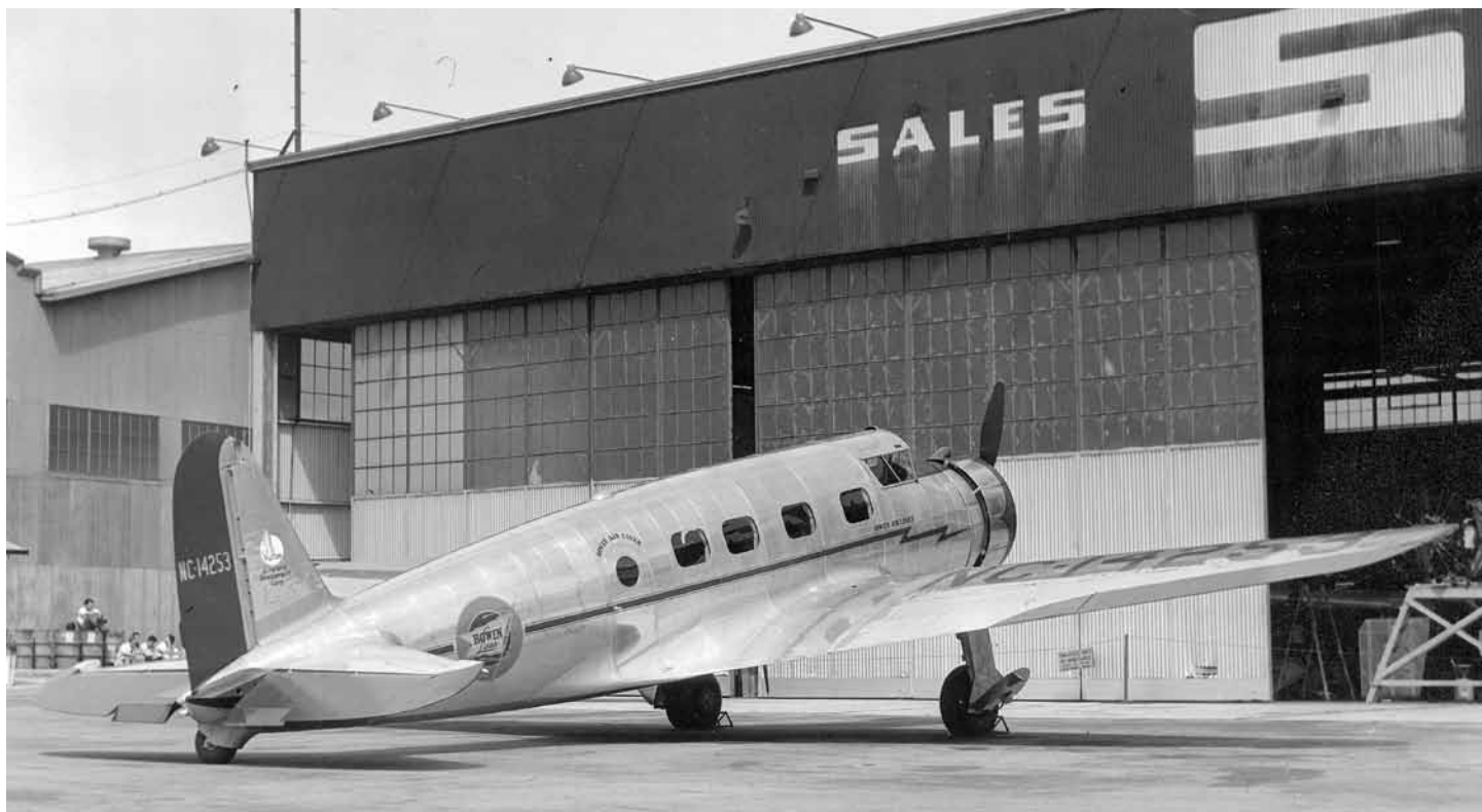
It is possible to see the thin panel sections that made up the V-1A's fuselage in this photo. This structural solution significantly reduced assembly time and maintenance costs. (Photo from the AAHS archives)
