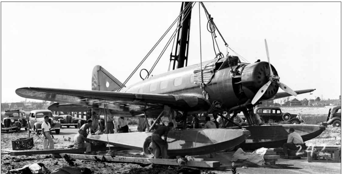
This Wright Cyclone GR-1820-GZ-powered Vultee V-1A was ordered by the Soviet Union in 1936. Equipped with EDO floats and a redesigned rudder assembly, it carried out its flight tests in the port of San Pedro, California. This seaplane, whose construction number is unknown, was registered CCCP L-208. (Photo from the Gerald Balzer collection, AAHS)
