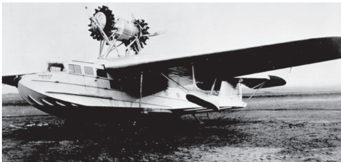
The Wright Cyclone engine, tried in both pusher and tractor arrangements still fell short on performance. Fokker attempted to fix the USAAC requirement with a tandem arrangement (similar to the F-32 engine pods) with two Pratt & Whitney Wasp engines. (American Fokker photo from the author's collection)
