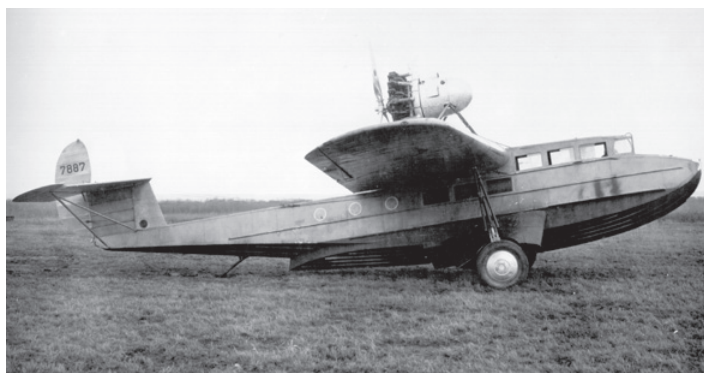
Initially configured as a flying boat, msn 901 would be modified into an amphibian with the addition of retractable landing gear. Note the abbreviated vertical stabilizer. This would be enlarged in future production versions. (American Fokker photo from the author's collection)
