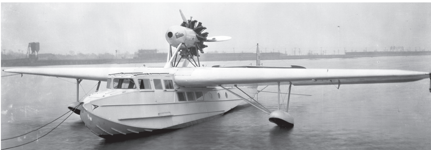
The sponson arrangement wasn't very successful and was soon removed, converting the prototype back to a flying boat. It was sold to Harold S. Vanderbilt as F-11 Special with a bigger wing and Cyclone engine. (American Fokker photo from the Boeing Company)
