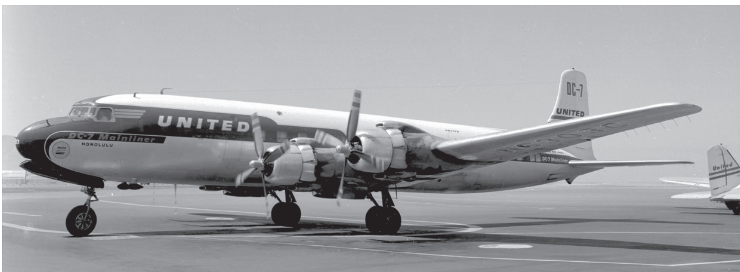
Early shot of a United Douglas DC-7 before spinners and inner cowl liners were added to aid cooling. United pioneered fleetwide radar installations shortly afterward. (AAHS photo archives, R. Hufford collection, AAHS-40102)
