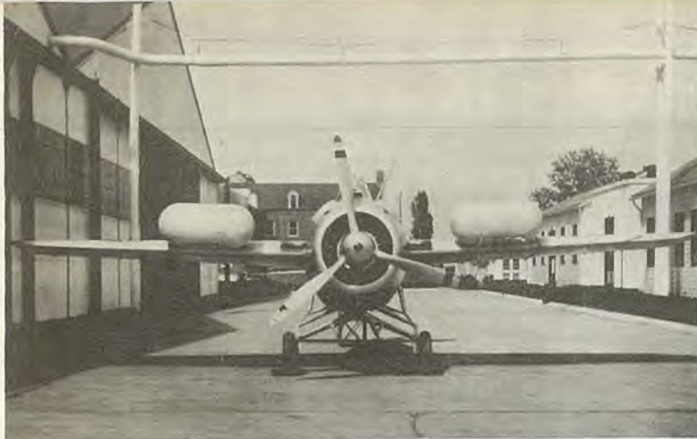
The XF4F-2 at Anacostia Naval Air Station, with flotation bags inflated. Photo - U.S. Navy No. 2833.
