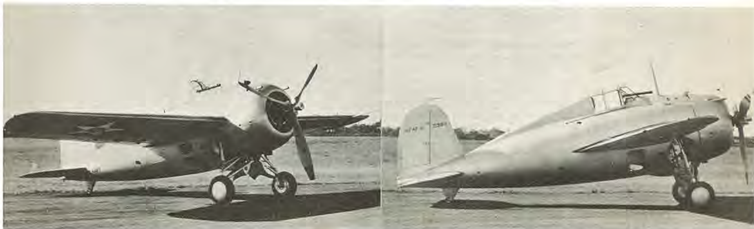
The XF4F-2, Grumman's first monoplane, followed the XF4F-1 Design No. 16, which was a biplane! The design of the biplane XF4F-1 is shown on Page 226. The pict-
