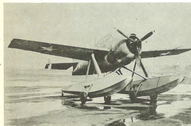
F4F-3, BuNo. 4038, with twin floats. Photo - Grumman No. P-926, 12-2-44.
