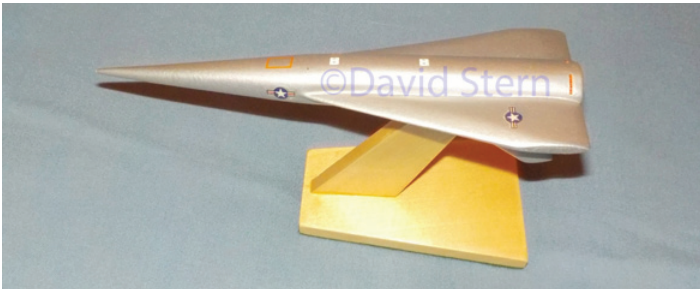
The final R459 Brass Bell reconnaissance glider configuration still undergoing refinements proposed to the USAF. Its clean top allowed a reasonable semi-recessed fit in an enlarged bomb bay of a Convair B-36 Mother-ship, also used to air-launched Bell Rascal missiles at Holloman AFB, New Mexico. (Photo & Model: Dave Stern).
