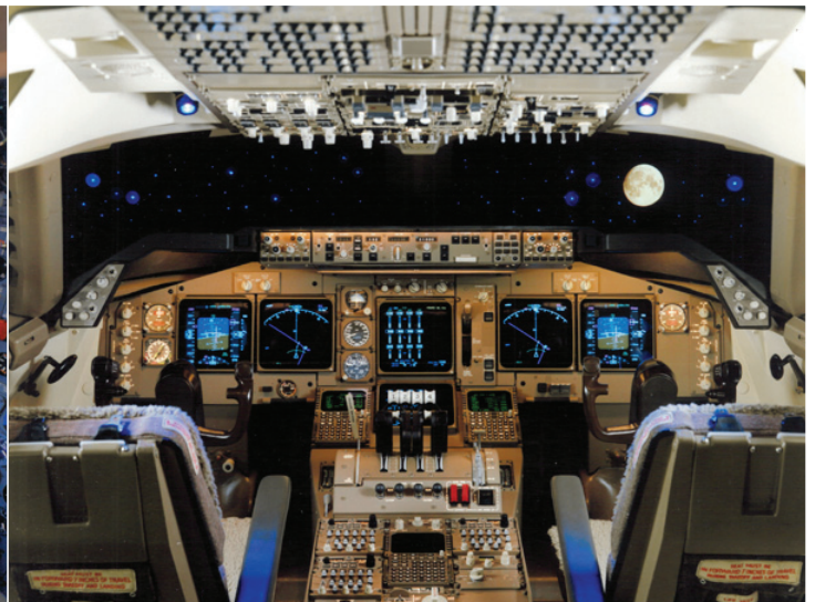
The 747-400's glass cockpit. Note the flight engineer's position has been eliminated. Automation has reduced the workload allowing the plane to be safely operated with just two pilots. (Photo from the Boeing Company)
