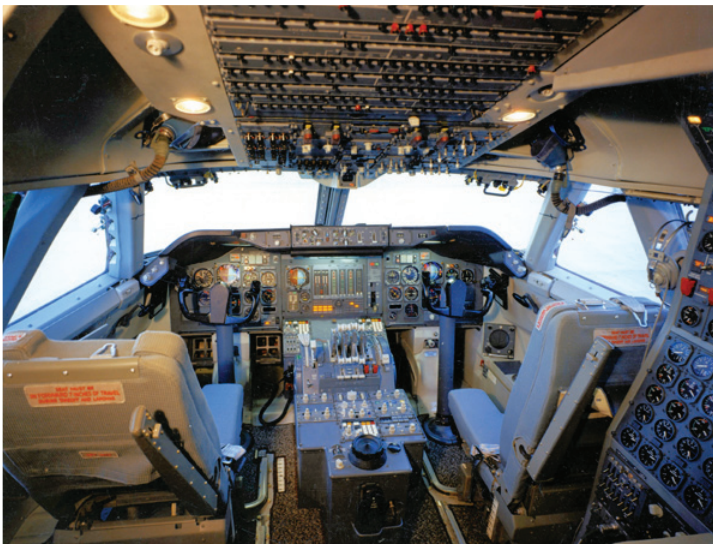
The 747-100's cockpit layout with "clockwork" gages. Note the flight engineer's position at the right side of the photo behind the copilot's seat. (Photo from the Boeing Company)
