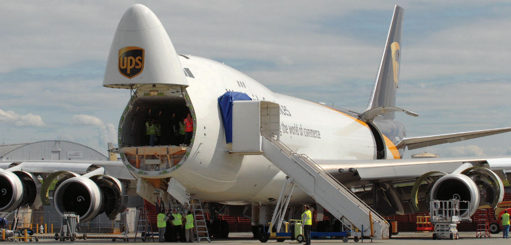
The upper flight deck stemmed from the anticipation that the 747 would eventually serve as a cargo carrier. (Photo from the Boeing Company)
