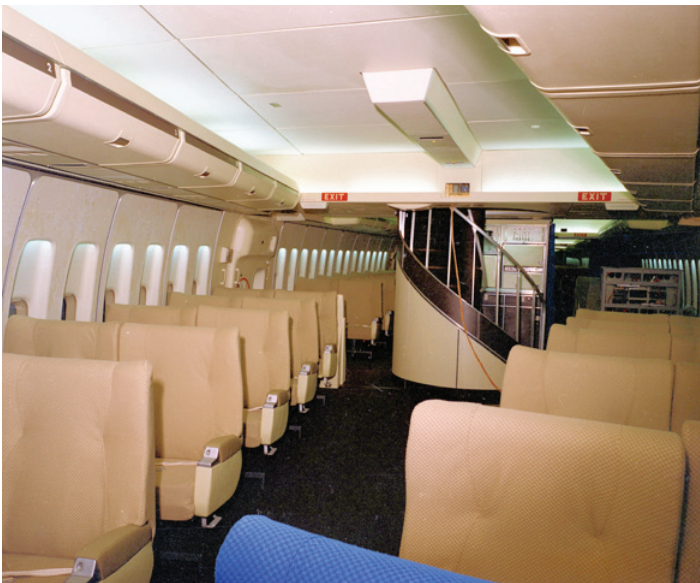
First Class (and later Business Class) passengers were forward of the main cabin entrance on the lower deck as seen here in PanAm's seating configuration for early 747s. (Photo from the Boeing Company)
