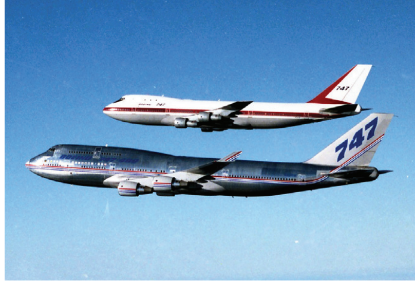
The extended upper deck and winglets on the Boeing 747-400 are easy differentiators of this series from the original 747-100. Seen here are the two prototypes flying in formation. (Photo from the Boeing Company)
