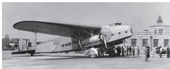
The 1930 version of a 747 wide-body, the Fokker 32 offered two-by-two seating. Capable of seating 32 passengers it often flew with less due to performance limitations. Here we see NC342N, c/n 1207 on a ramp waiting to board passengers. (Photo from the Gerald Balzer collection, AAHS archives)
