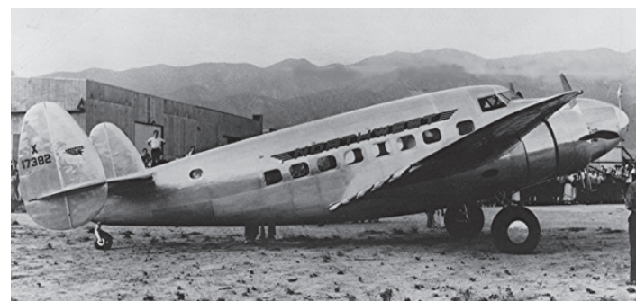
First Lockheed Super Electra before aerodynamically balanced rudders were installed (Lockheed photo from the author's collection)
