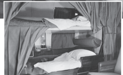
DST accommodations were first class. Here we see the convertible seating arrangement in both seating and bunking configurations. (American Airlines photo from the Glenn Moss collections, AAHS archives)
