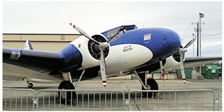
Boeing 247 owned by the Seattle Museum of Flight and restored in the overall paint adopted by United to cover the original dull gray anodized finish. Note the original forward-sloping windshield. (Photo from the author's collection)
