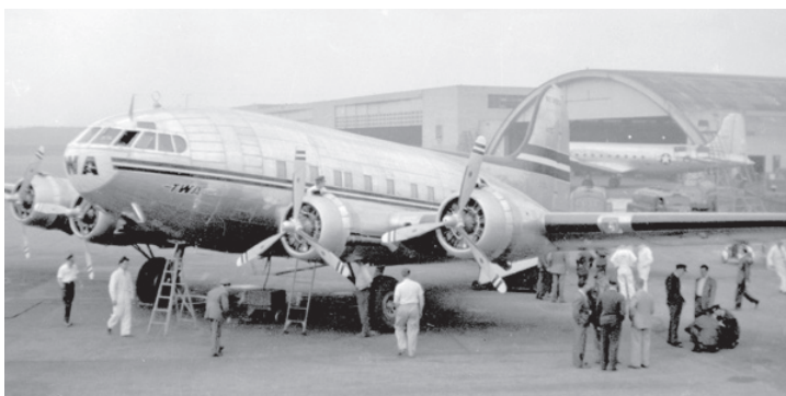
TWA Boeing 307B, N19903, c/n 1999, being prepared for its next flight. This is a postwar photo after TWA's planes had been completely rebuilt by Boeing with surplus B-17G wings, engines & other components (Al Eldridge collection from the AAHS archives, AAHS-52762)
