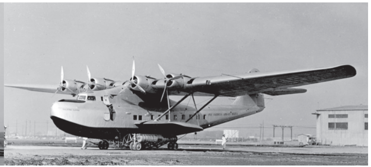
This view of Pan American Martin 130 Philippine Clipper, NC14715, c/n 557, clearly shows the raised cabin cross-section that provided a more aerodynamic wing-fuselage configuration. (AAHS archive, AAHS-D020825)
