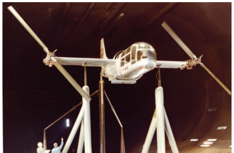
Figure 15: XV-3 tiltrotor aircraft in the NASA Ames 40-by 80-foot wind tunnel (Ames photo A-37006-5)
