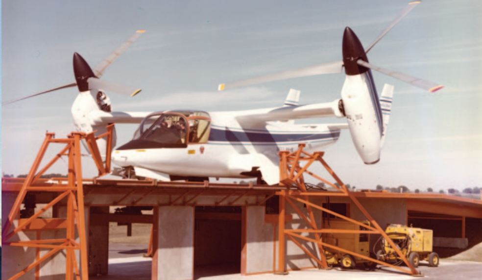
LEFT - Figure 25: Simultaneous static test firing of ejection seats. (Ames photo AC75-1602) RIGHT - Figure 26: Ground tie-down test facility at Bell's Arlington, Tex., Flight Test Center. (Bell photo 304932)
