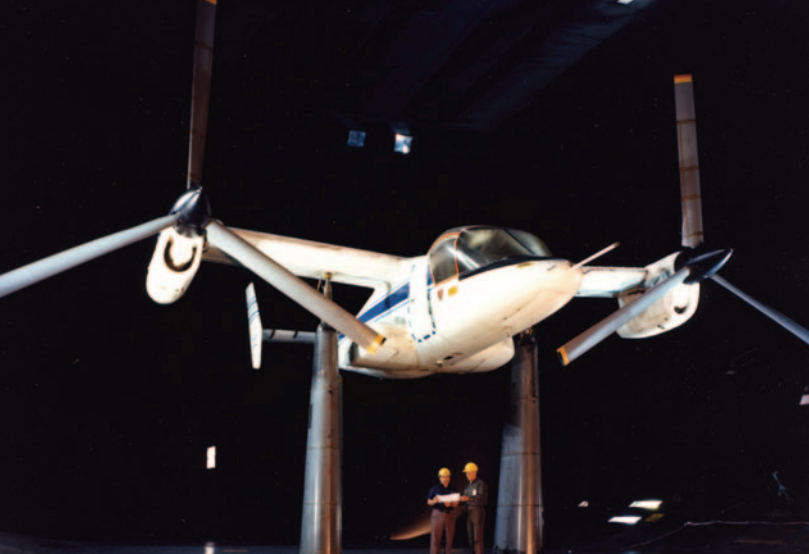
Figure 27: XV-15 tiltrotor research aircraft in the NASA Ames 40-by 80-foot wind tunnel. (Ames photo AC78-0579-3)
