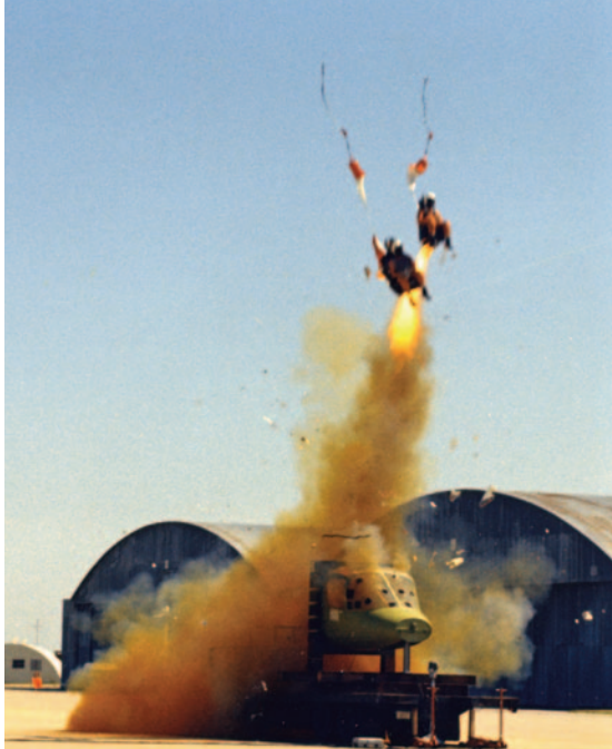
LEFT - Figure 25: Simultaneous static test firing of ejection seats. (Ames photo AC75-1602) RIGHT - Figure 26: Ground tie-down test facility at Bell's Arlington, Tex., Flight Test Center. (Bell photo 304932)
