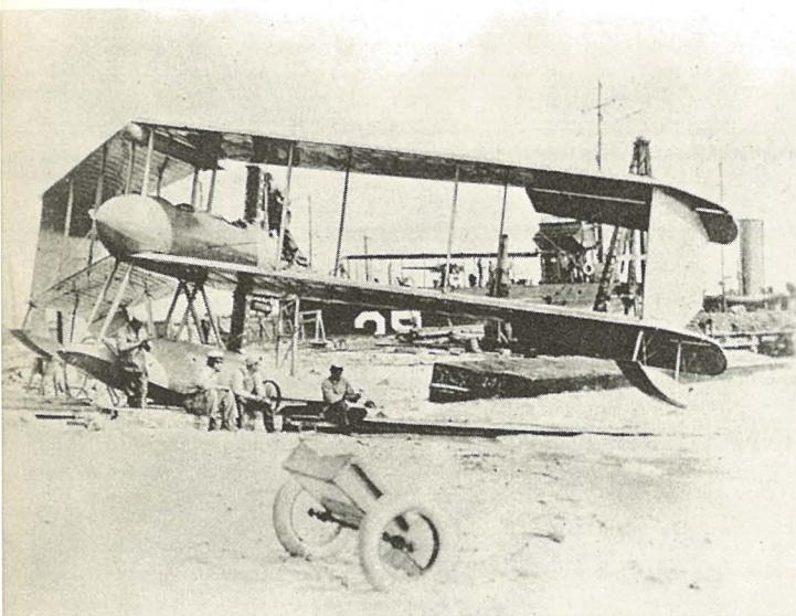
Below - A modified Curtiss N-9 seaplane (150 HP Hispano-Suiza/Wright-Martin built engine, large spinner, wing mounted radiator) used in catapult tests aboard the U.S.S. OKLAHOMA. (Photo - U.S. Navy #428435)
