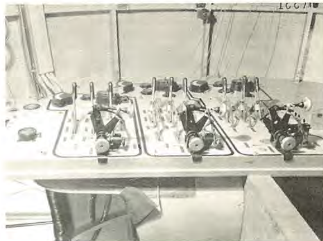
7. The observer's panel, to right of pilot, was poorly arranged, with some controls moving horizontally, others vertically. (Photos - McCook Fd. Nos. 16667 & 16670 respectively, from Air Force Museum.)
