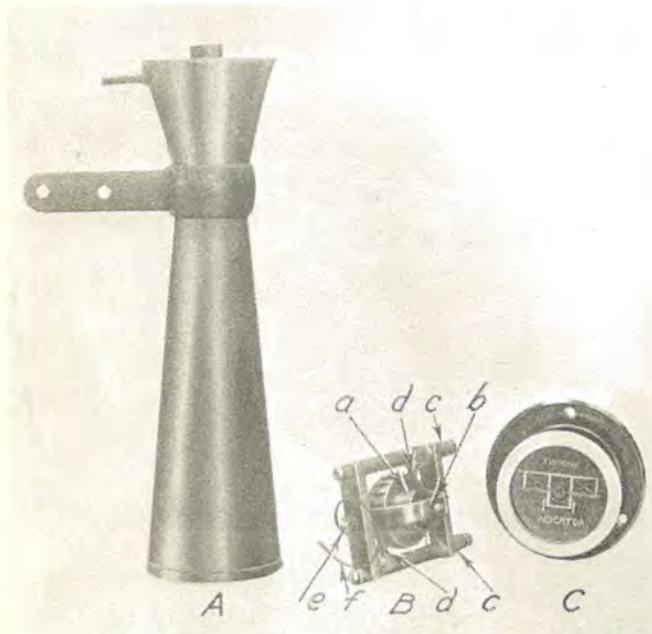
3. The first pictorial display of an aircraft shape on the face of an instrument to show aircraft attitude. This was introduced by Sperry in 1919. (Photo - A.F. Museum)
