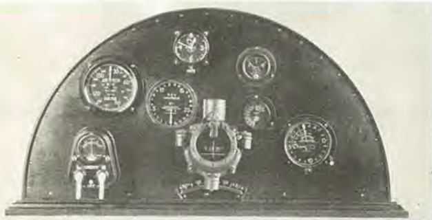
4. Panel of production type DH-4. In Photo No. 5 at right is shown the advanced design panel installed in
