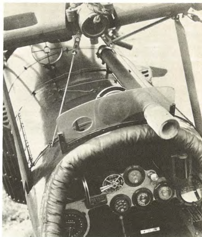
Panel of Orenco PW-3, 1921. Compass was located in wing and airspeed indicator in front of windshield. (Photo - McCook Fd. #10311, Air Force Museum #N58-D1-195)
