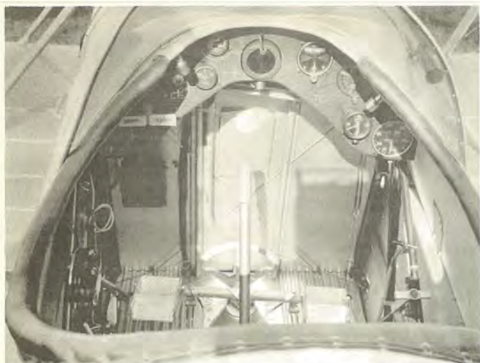
10. Instrument panel of Boeing Model 40A Mailplane. (Photo - United Air Lines.)
