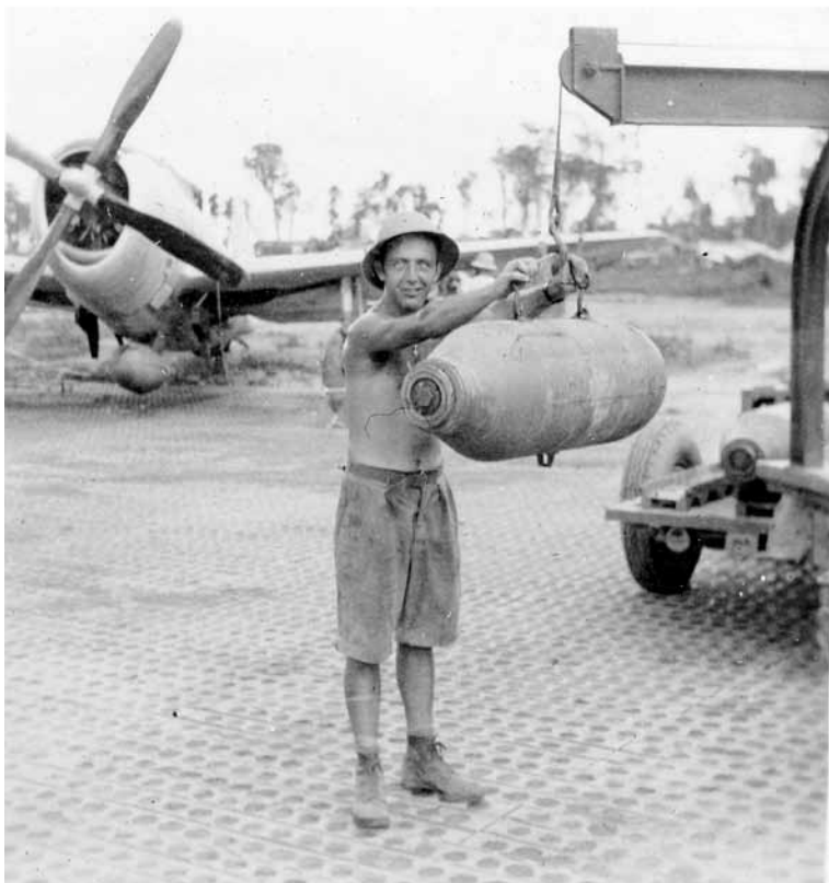
LEFT: This armorer is hauling a bomb with a crane to attach it the P-47 behind him. The parking areas and taxiways at Moran were made with Pierced Steel Planking (PSP). ABOVE: These armorers are attaching a 250-lb bomb under the wing of the P-47. The detonator is not installed yet.
