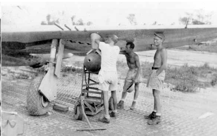
LEFT: This armorer is hauling a bomb with a crane to attach it the P-47 behind him. The parking areas and taxiways at Moran were made with Pierced Steel Planking (PSP). ABOVE: These armorers are attaching a 250-lb bomb under the wing of the P-47. The detonator is not installed yet.
