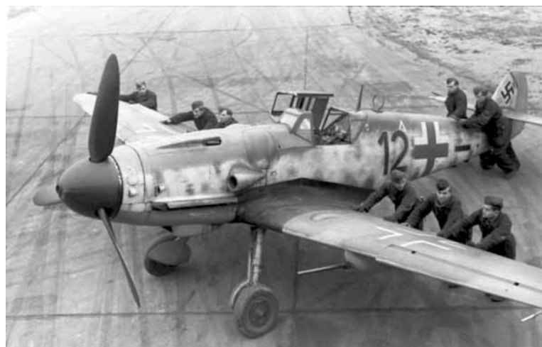
Luftwaffe ground-crew ("black men") positioning a Bf 109 G-6 "Kanonenvogel" equipped with the Rüstsatz VI underwing gondola cannon kit. Note the slats on the leading edge of the port wing. JG 2, France, late 1943. (From the author's collection)
