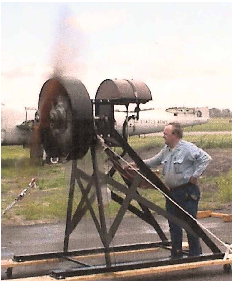
The author, and chief mechanic for the project, during a test run of the restored Gnome Omega engine. The engine has been test run a total of more than 36 hours. (Photo from the author)
