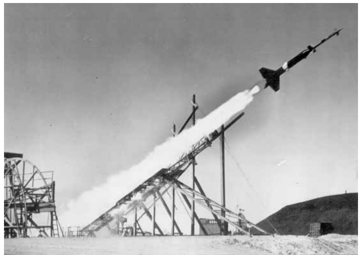
The Bell air-to-air Meteor missile project. The missile was air launched from a Douglas F3D Skynight test aircraft but also ground launched with a booster rocket shown here. Other than their XS-1 rocket research aircraft, the Meteor was their first post war rocket powered missile project. (Bell photo)
