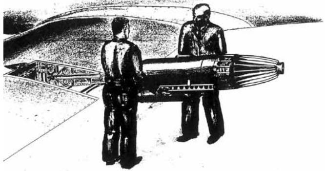
Bell drawing of the rocket motors projected for installation on their Army Air Corps Model 3 interceptor. The Model 3 morphed through redesign with the cockpit moved forward and a liquid-cooled Allison engine behind it, to become the P-39 Airacobra fighter. (From the AAHS collection)
