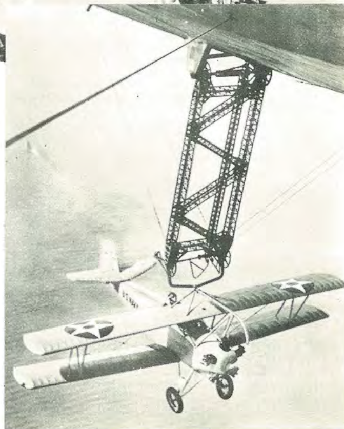
The Vought OU-1 is prepared for static test of the sky-hook at the Naval Aircraft Factory. This photo is from N.A.F. Technical Report No. 718, dated 10 July 1928. The alphabetical keys were on the original print. See box on Page 97 for technical description of its operation.
