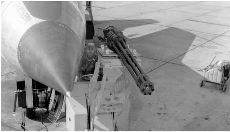
An F-105's Vulcan 20mm cannon being serviced. (Photo from the AAHS archives, AAHS-D024159)
