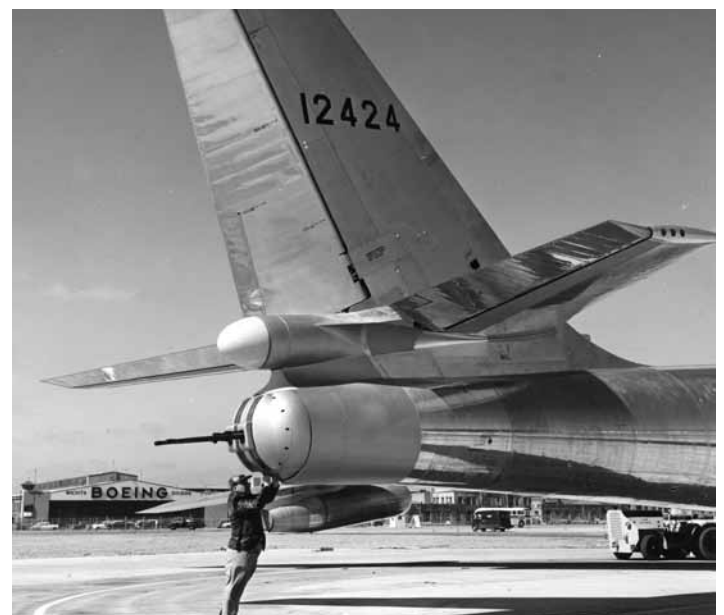
The stinger end of the Boeing B-47 with weapon radar in the pod just above turret. (Photo from the AAHS photo archives, AAHS-D022535)
