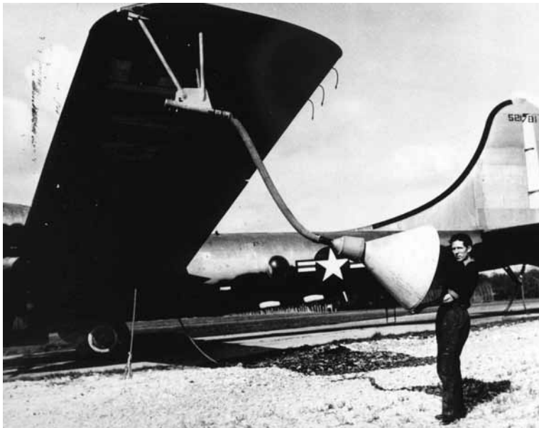
To evaluate the behaviour of a drogue trailed from the wingtip of a B-29, a short length of hose with drogue was fitted to the LRF receiver 45-21781 for flight tests. (FRL neg 950)
