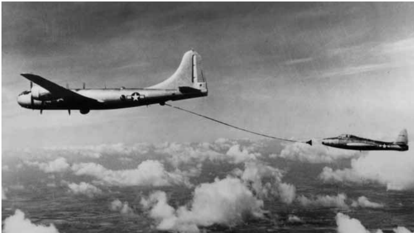
Seen here over the south coast of England, the single-point B-29 tanker 44-69704 refuelled Schilling west of Greenland but Ritchie was unable to take on fuel because of a stuck nozzle valve. (USAF photo, 39655 AC)
