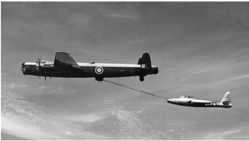
Lincoln RA657 was used in RAF evaluation trials and permission was given for it to be used in the Fox Able 4 flight to refuel the F-84s over Iceland. (Copyright Charles Brown Collection, RAF Museum, ref 6421-1)
