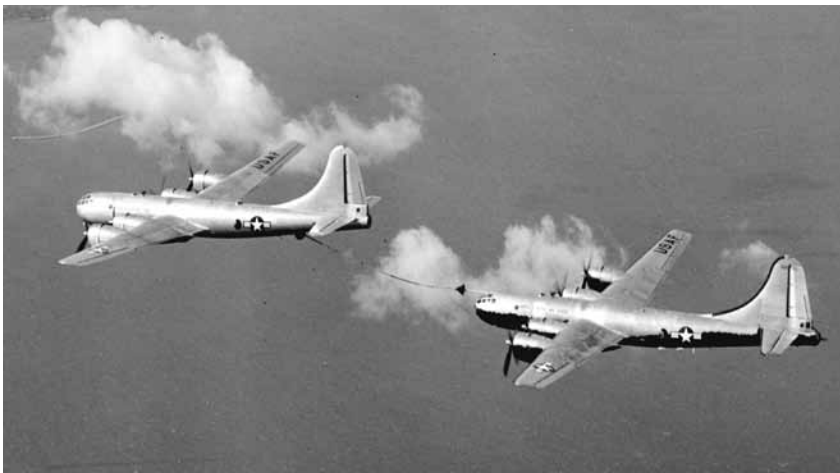
The Low rate of flow (LRF) B-29 receiver (45-21781) in contact with the single-point tanker (44-69704). The greatest amount of fuel transferred during continuous transfer was 4,120 U.S. gallons at an altitude of 8,000 feet and the receiver system functioned satisfactorily at all rates of flow between 150 and 260 US gpm. (Copyright Charles Brown Collection, RAF Museum, ref 6422-3)
