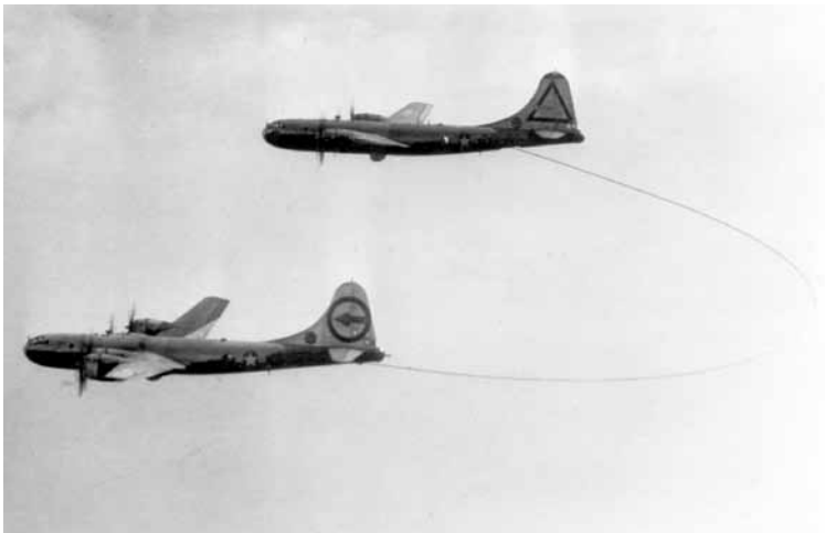
A KB-29M (upper) refuelling a B-29M with the 'looped hose' system. (USAF photo 253630 AC)
