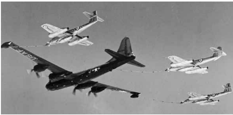
Simultaneous three-point refuelling demonstrated by the YKB-29T with two Meteor F.8s from 245 Squadron RAF and the FRL Meteor IV VZ389. (Copyright Charles Brown Collection, RAF Museum, ref. 6446-7)
