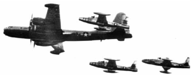
During tests in the U.S., the YKB-29T demonstrated simultaneous refuelling with two probed F-84Es and a T-33A with probed tip tanks (representing an F-80). This tanker was subsequently modified by Hayes Aircraft Corp. to have U.S.-built A-12B refuelling units in place of the original British equipment. (USAF Museum photo)
