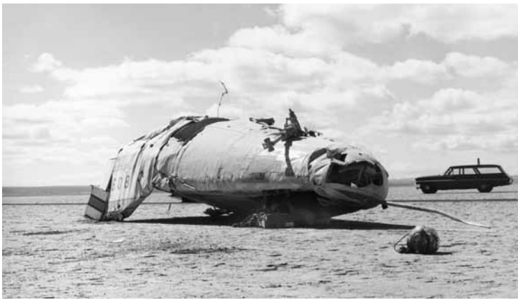
Figure 16. The M2-F2 on Rogers Dry Lake after its crash on May 10, 1967. (Photo from NASA, FRC E-16731)
