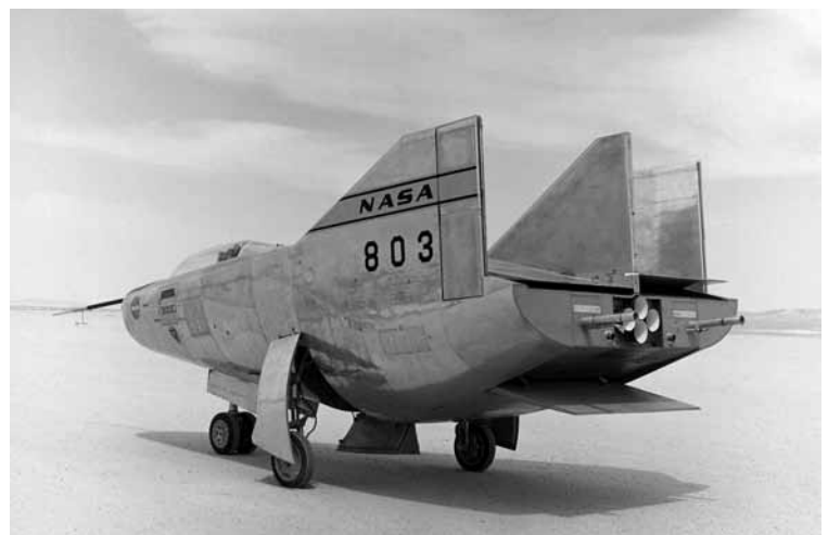
Figure 18. The M2-F3 is shown on Rogers Dry Lake with the XLR-11 rocket engine installed. (Photo from NASA, FRC E-21533)
