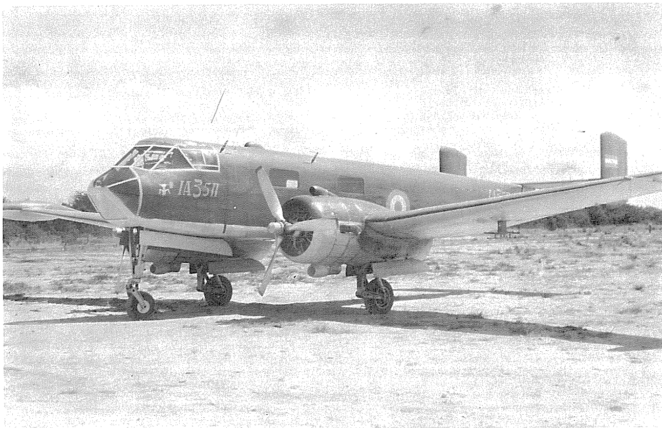
FABRICA MILITAR de AVIONES 1A-35-II "Hanquero" Light Transport. An S.I.A. photo. The "Hanquero" is now produced in three versions, the -Ia and -Ib Crew Trainers, and the -II Light Transport. The latter are occasionally used by Argentine Army airborne troops, and the -Ia and -Ib are in service with the Fourth Air Brigade.
