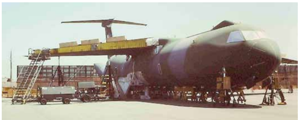
67-0029 undergoing a wing replacement at Iwakuni AB. The inner portion of the right wing would be crated and sent to AMARC for storage. (USAF photo provided by Dave Grant) 15
