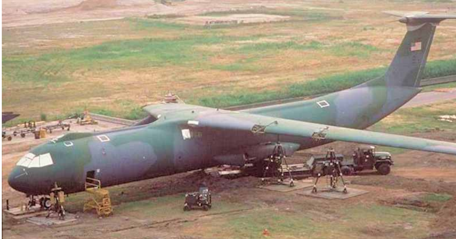
The weight of the aircraft is almost off the wing jacks and onto the truck trailer. (USAF photo from the D. Grant collection) 9
