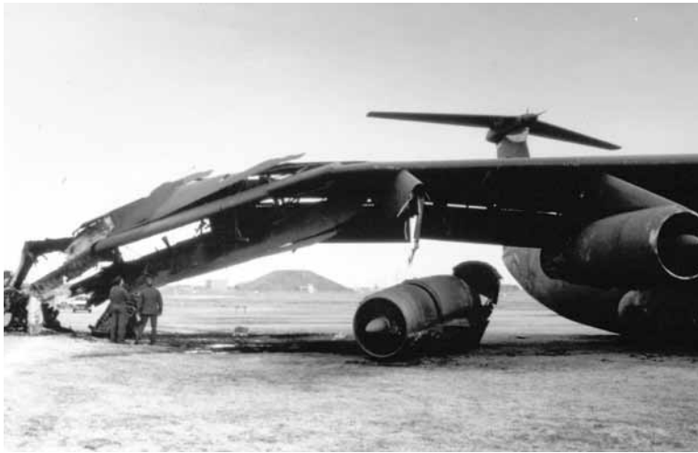
The damage to the right wing and no. 4 engine was extensive. 7 (USAF photo)
