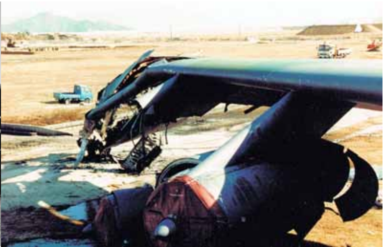
Note the thrust reverser on no. 3 engine is still deployed. (Photo from the Paul Minert collection)
