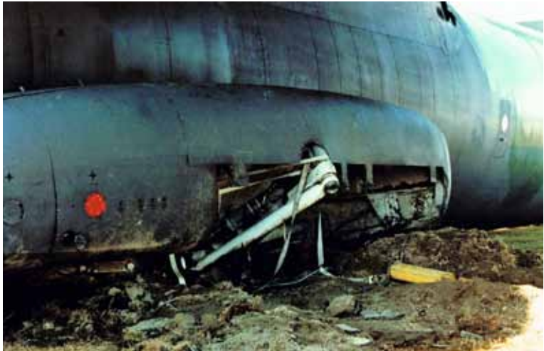
The extensive damage to the right main landing gear assembly is evident in this photo. (Photo from the Paul Minert collection)
